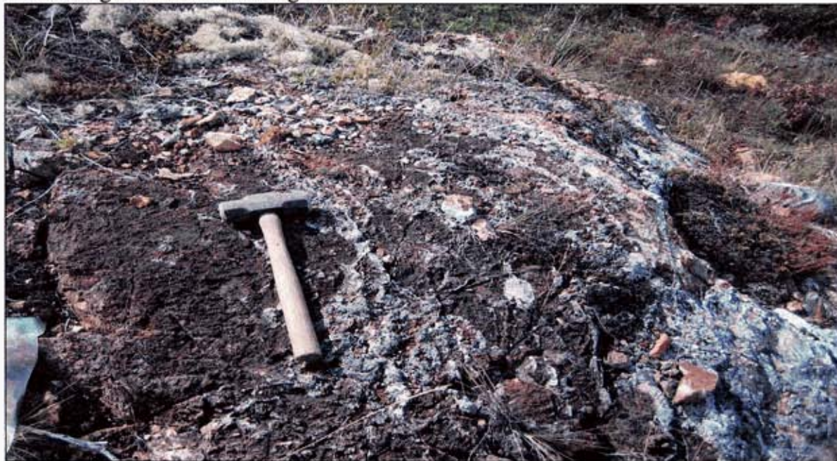
Pictou Area, Atlin Airport; Altered Harzburgite: Alteration: Carbonatized-Quartz-Fuchsite; stringers of Quartz
