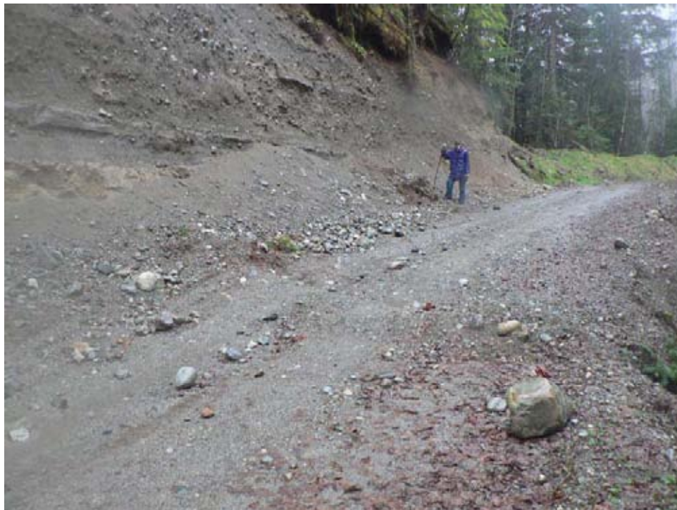
Figure 8b : Statlu South – Central Area unit 3 gravel sitting on top of unit 2 silt-sand
