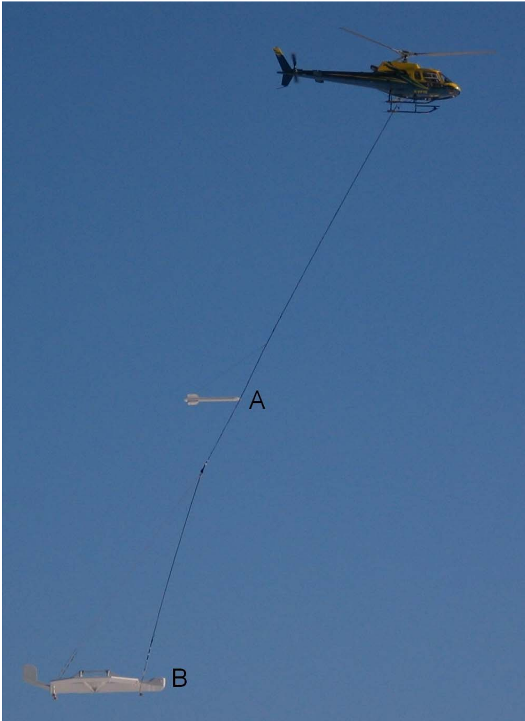
Figure 4. The magnetometer bird (A) and AeroTEM II EM bird (B)
