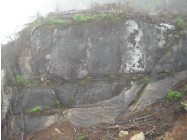
Photo 74 – Semi massive intrusive. Fracture pattern suggest blocks in the order of 200 to 600 tons.
