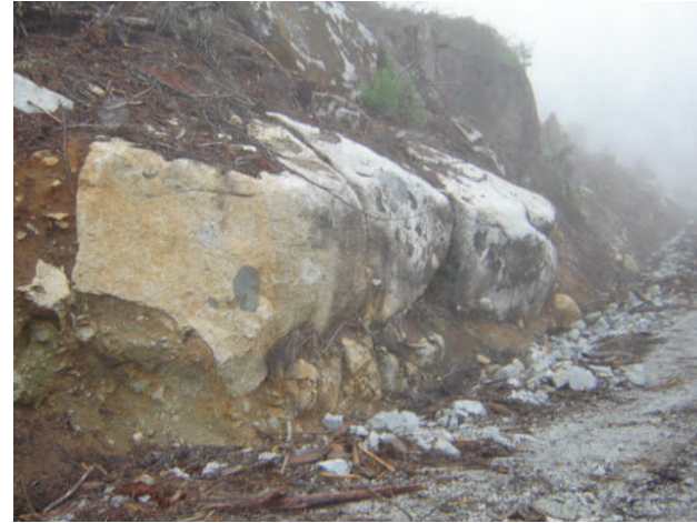
Photo 75 – Large blocks of intrusive. Note large xenolith in exposed face. Limonite stain is only a surface feature and does not extend into the stone.
