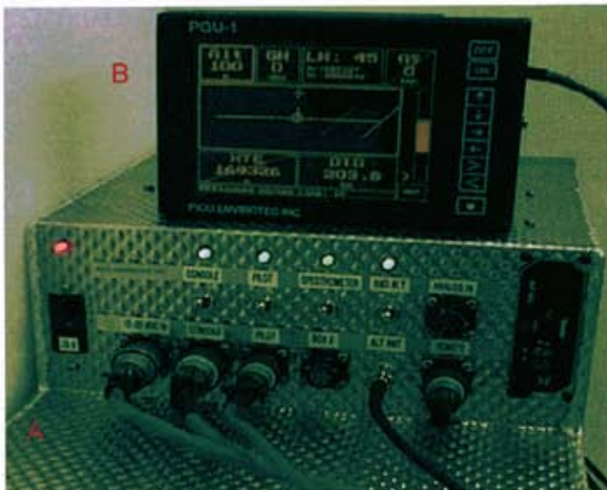
Figure 6. Aeroquest AGRS system. A. AGRS Sensor (Crystal Pack), B. Data acquisition computer.
