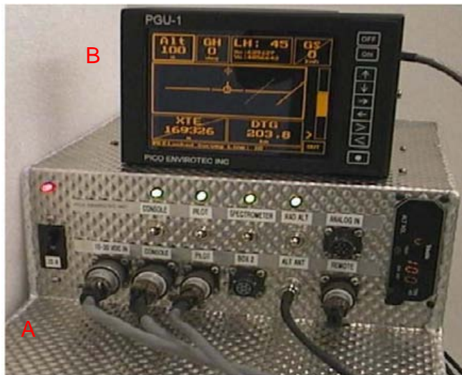
Figure 7. Aeroquest AGRS system. A. AGRS Sensor (Crystal Pack), B. Data acquisition computer.
