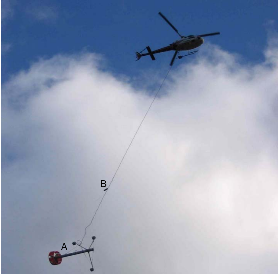
Figure 6. The gradiometer bird (A), and GPS antenna (B). The AGRS system is located in the helicopter cabin.
