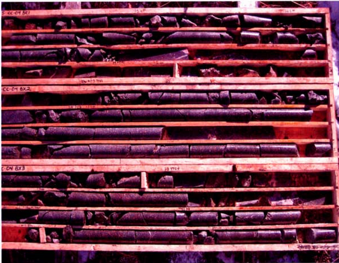
Box 1 -3, Interval 3.05 m -18.55 m. The dark brown to brown porphyritic andesite is characterized by a Fe enriched matrix, which is a result of the propylitization process, and hypidiomorphic feldspar crystals floating in the dense to fine grained matrix.
