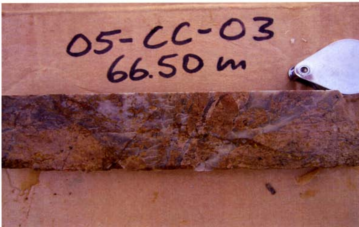
Close-up of stock work veining. Multiphase mono-mineralic (quartz) veins are replacing partially andesitic host rock and filling open fractures in a syn-tectonic event.
