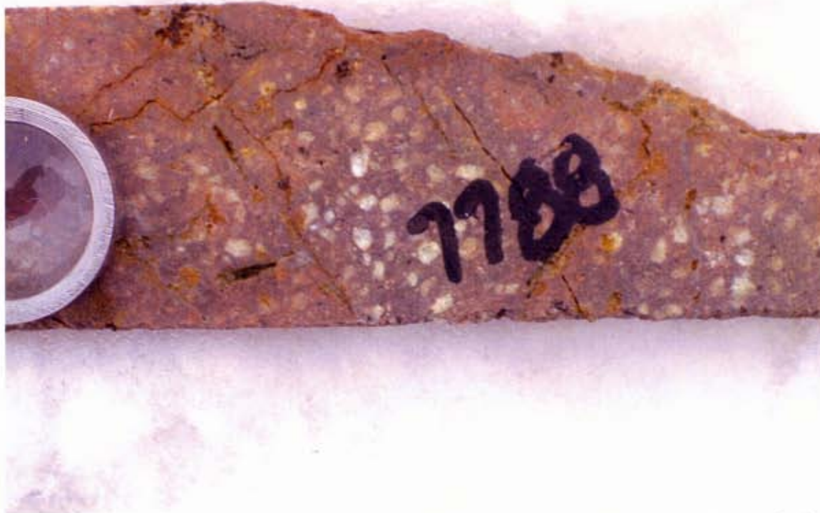
Close-up of a portion of sample 7788, 32.00 m – 33.00 m. The plagioclase crystals in the oxidized matrix of the porphyritic andesite are kaolinitic. The rock shows weathering related fractures and vugs.
