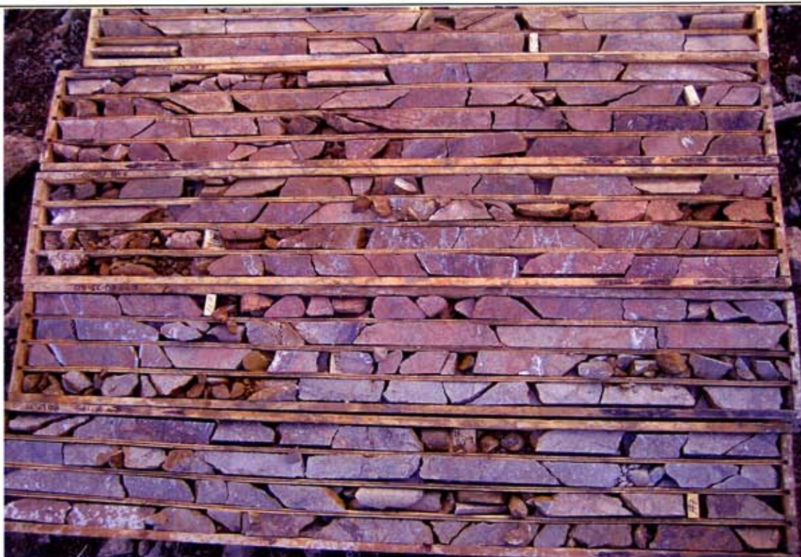
Boxes 5 - 8. Interval from 23.94 m – 46.36 m. Highly silicified limonitic to hematitic porphyritic andesite in the oxidization zone with stockwork veining + collapse breccias.
