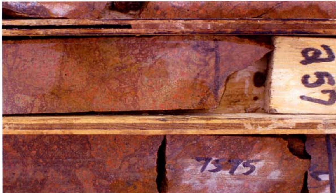
Fragmented and metasomatically altered and strongly silicified clasts of a hematitic, porphyritic andesite @ a depth of around 77.00 m in hole 05-CC-02.
