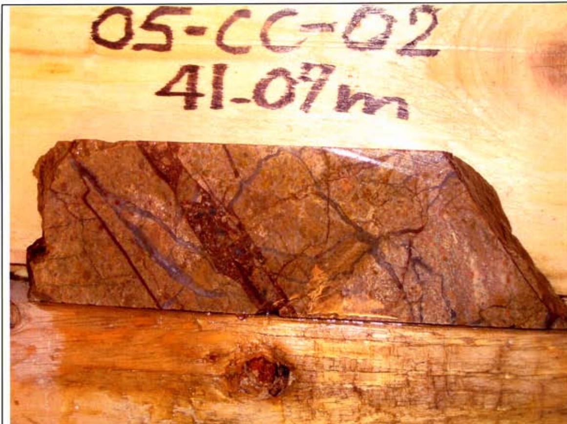
Close-up of stockwork veining. Multi-phase quartz veins, some are zoned and a late stage Open-fracture-filling by a hematitic-quartz narrow collapse breccia with altered, angular wall rock fragments. Piece of core shows still the weathering influence by its limonitic hematitic colors. Vertical depth below surface is around 22 m.
