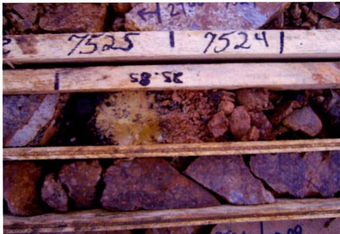
Fault zone @ 25.85 m depth. Limonitic, pyrolusitic clay in a porous and vuggy stock-work zone.
