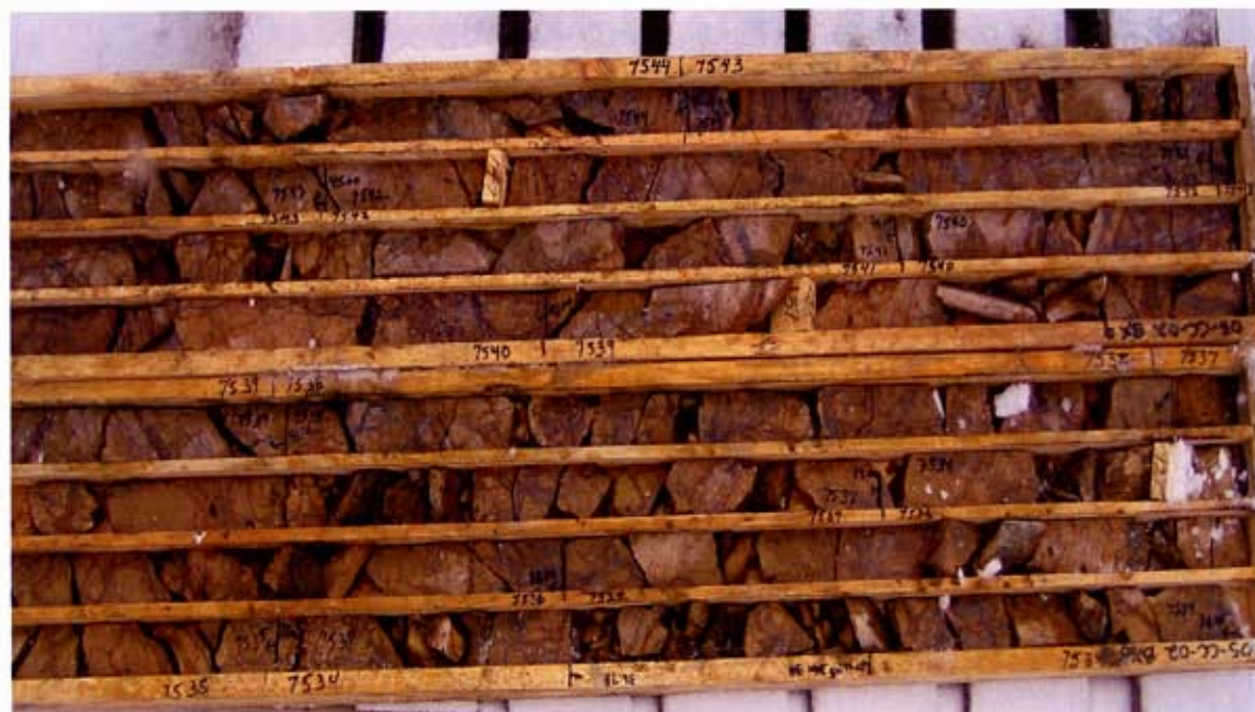
Box 8 + 9, Interval 36.00 – 51.47 m . Extensive stockwork multi-phase, poly-mineralic veins, often zoned replacing the porphyritic andesite.
