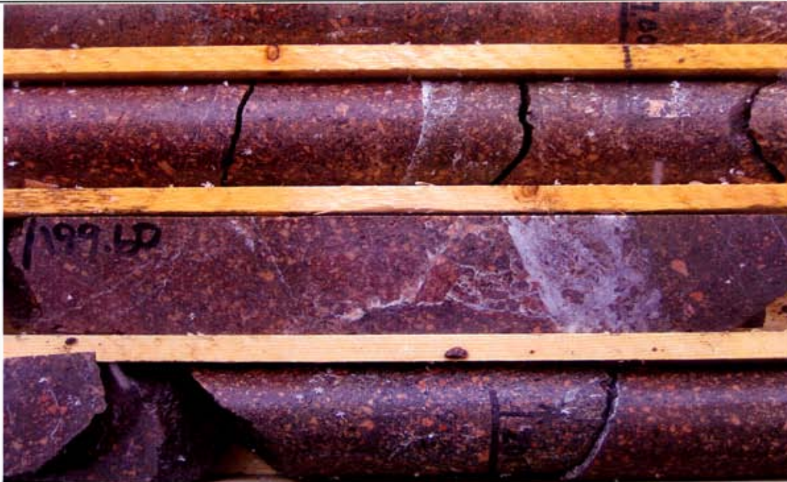
Close-ups of a calcite-quartz-siderite vein with wall rock fragments at 199.60 m depth.
