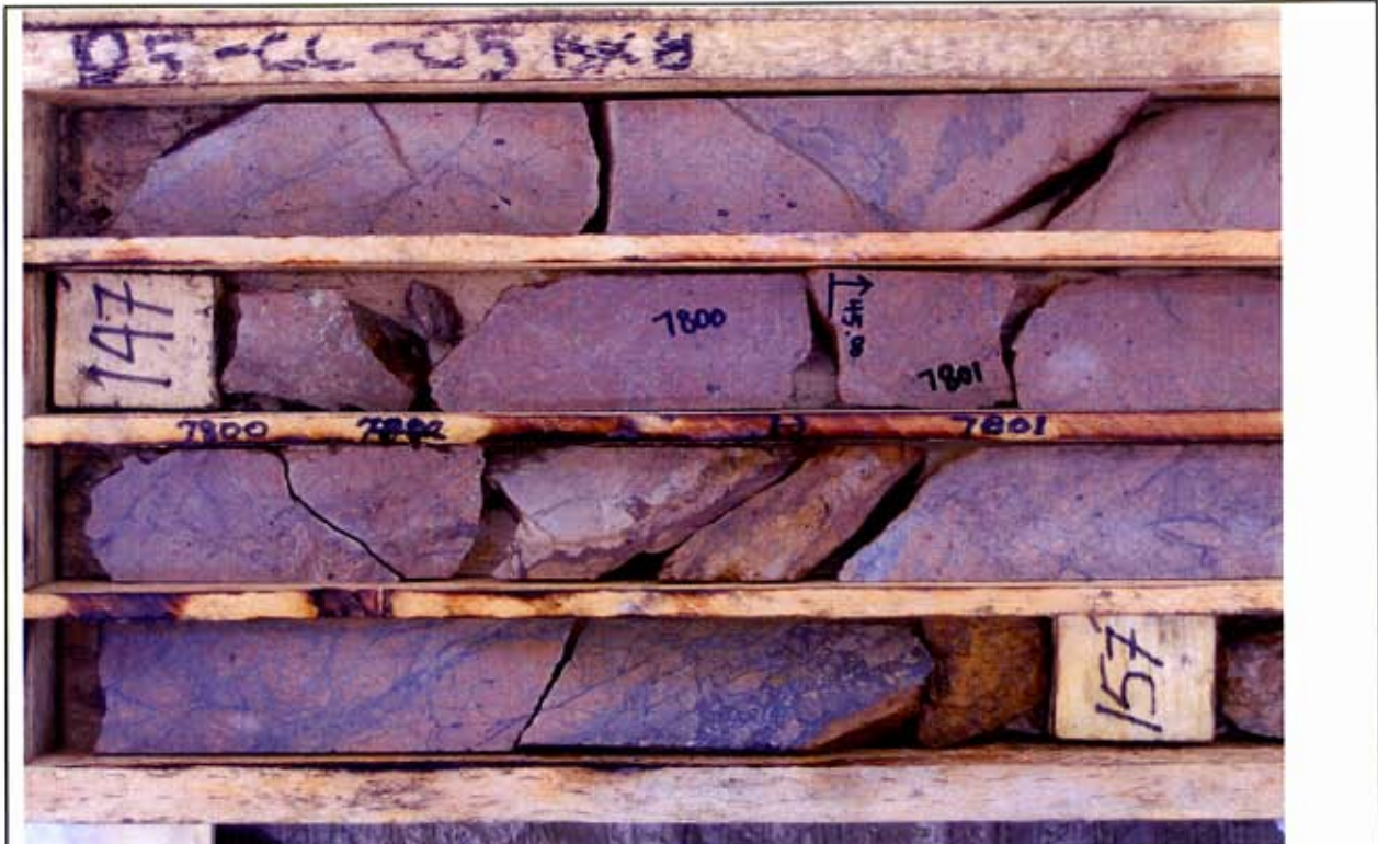
Close-up of a portion of hole 05-CC-05. Oxidization zone and brecciated andesite. End of hole at 174 feet in the upper portion of a strongly mineralized stockwork zone. Assay results show high gold and silver values, indicating the beginning of a gold-silver mineralized zone.
