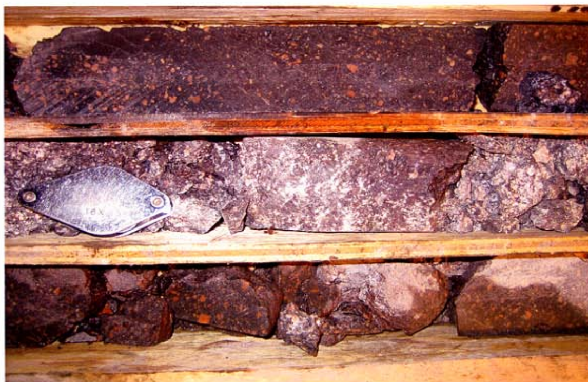
Close-up of porphyritic andesite with alauin (?) at a depth of 146.68 m at magnifying lense. The aphanitic matrix has a hematitic brown color, which is common due to the propylitization of the andesite.
