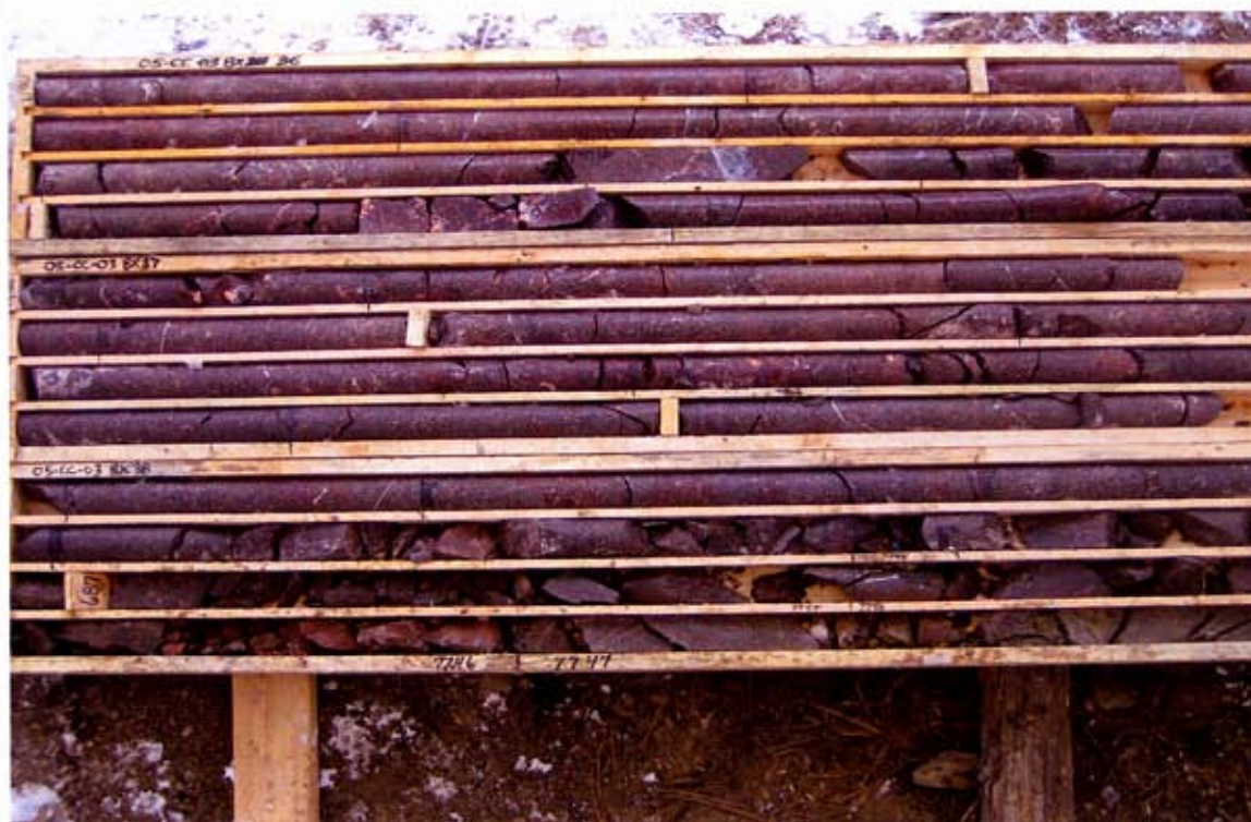
Hole 05-CC-03, Box 36 - 38, Interval 168.21 m - 211.80 m. Again a post mineralization event fault zone.
