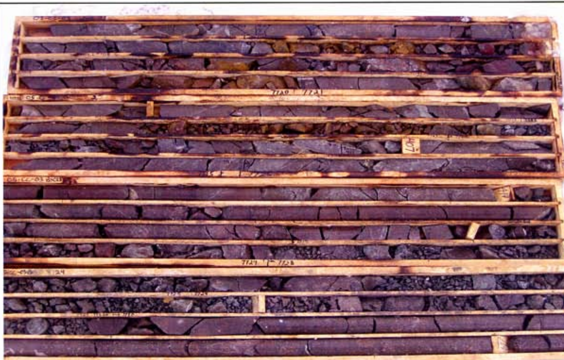
Hole 05-CC-03, Box 21 – 24, Interval 115.37 m – 136.44 m. Lower box in photo shows brittle deformation. A late stage fault in the andesite.
