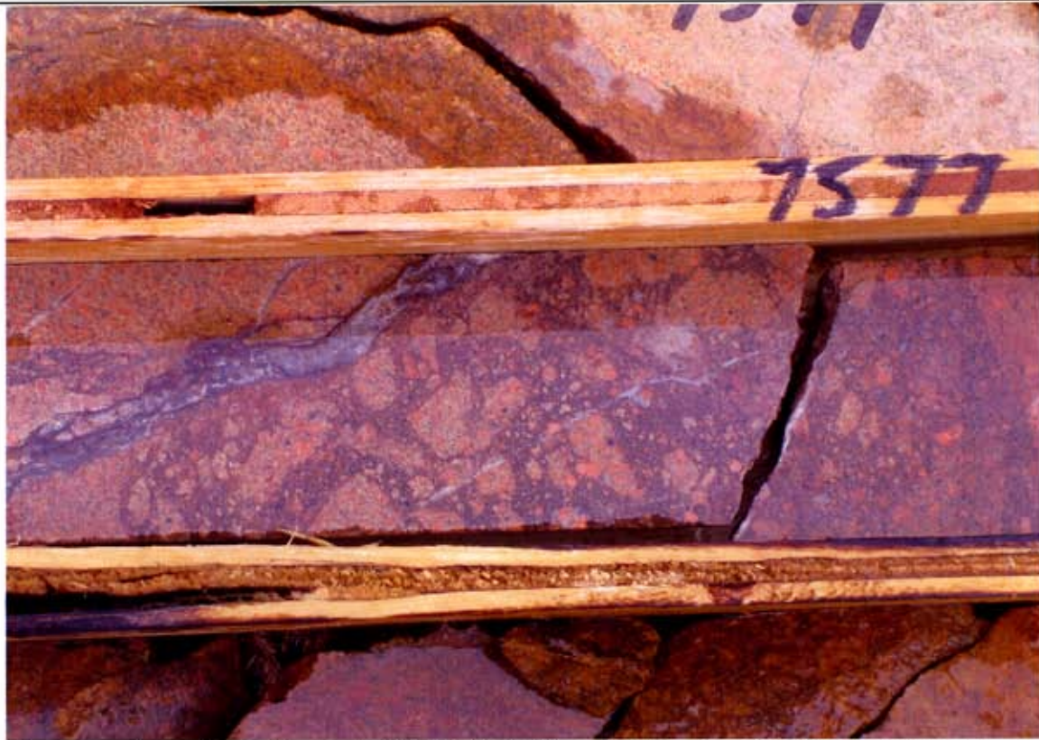
Close-up of a portion of sample #7577 @ 79.00 m depth is showing brecciated (collapse breccia ?) porphyritic andesite cut by narrow late-stage quartz veins.
