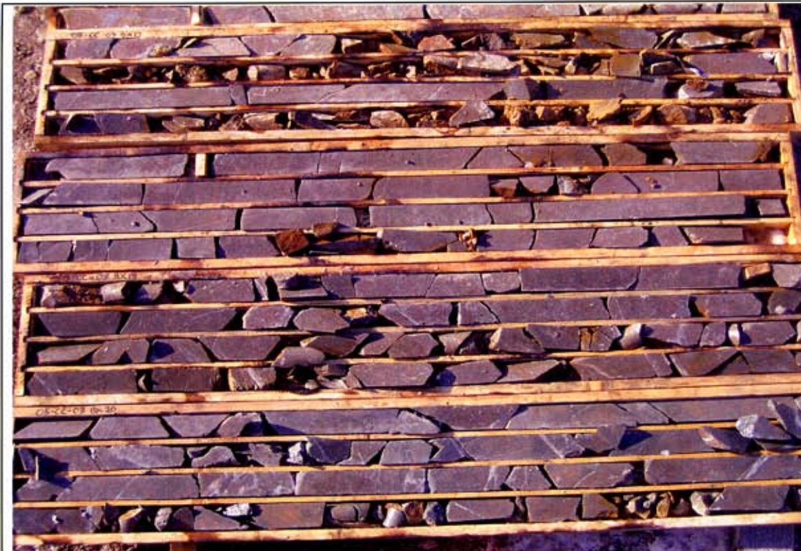
Hole 05-CC-03, Box 17 – 20, Interval 94.75 m – 115.37 m. Porphyritic andesite with qtz-veins in the hanging-wall of the stockwork veining.
