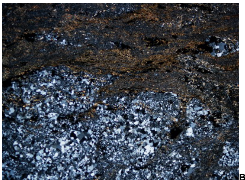
Hen 941 – 69.5: Representative view showing bands of quartz, biotite, K-feldspar and sulfides FOV = 8.5 mm, A) PPL, B) XPL
