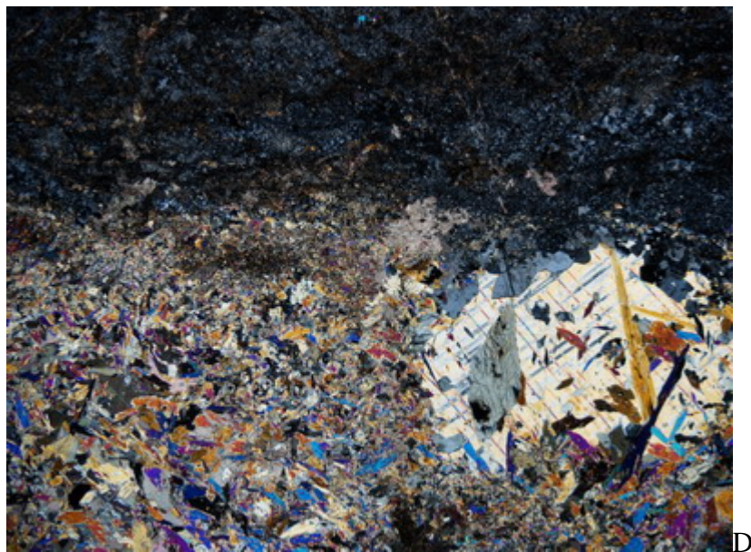
Hen 941 – 69.5: C) Representative view showing bands of arsenopyrite (white) and pyrrhotite (pinkish). FOV = 8.5 mm, RL. D) Representative view of a different area in the sample. The top are bands of quartz and biotite, while at the bottom the sample is made essentially of carbonate and laths of actinolite-tremolite, FOV = 8.5 mm, XPL
