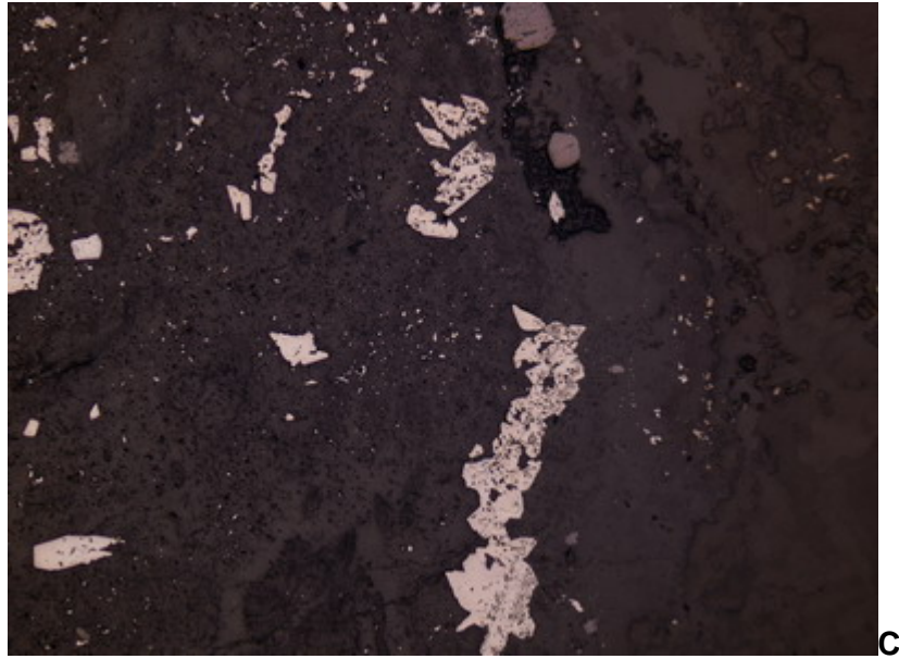
Hen 92 – D3: C) same view as above showing disseminated and stringer arsenopyrite (light grey) with minor ilmenite (dark grey). FOV = 8.5 mm, RL
