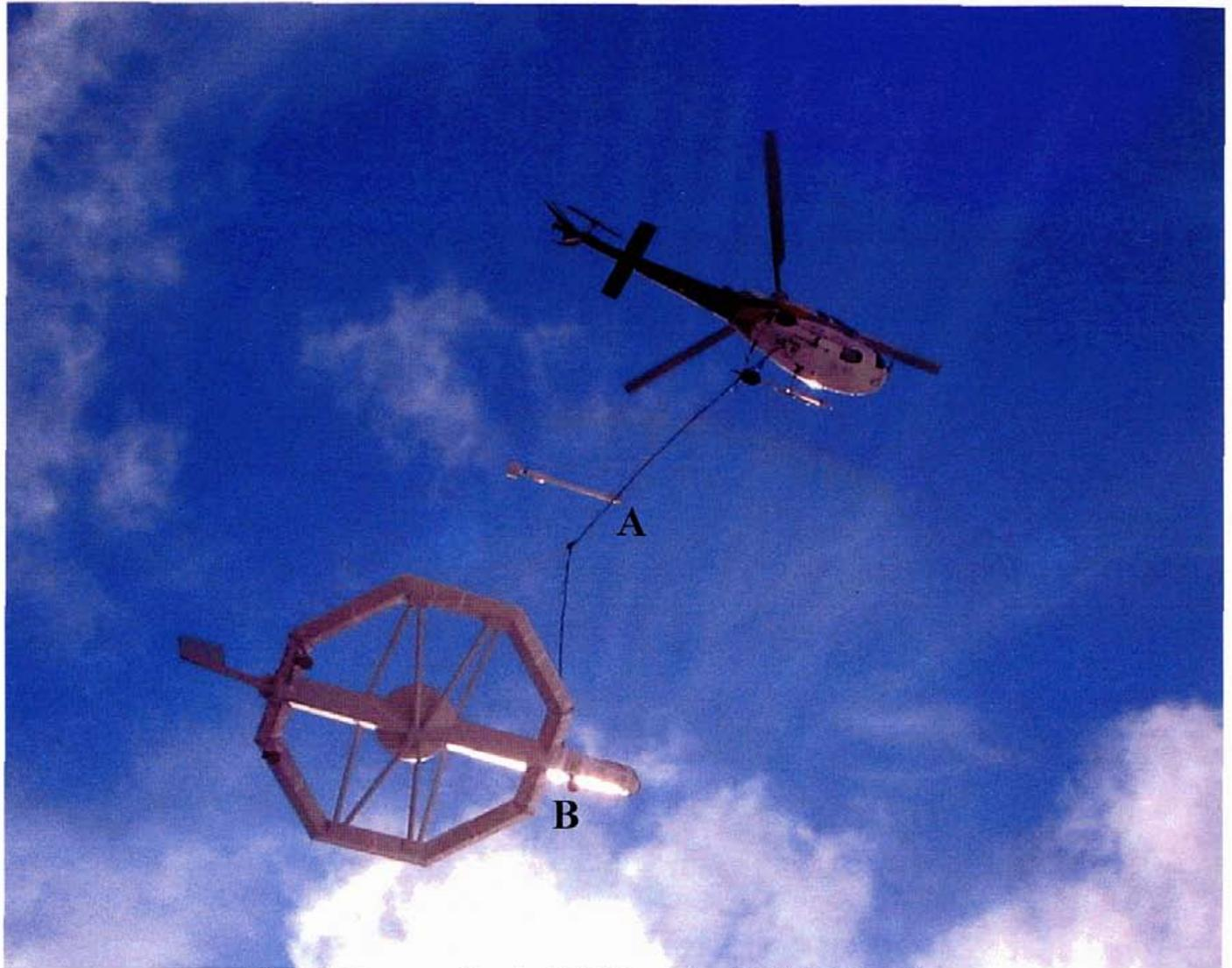
Figure 4. The magnetometer bird (A) and AeroTEM II EM bird (B)
