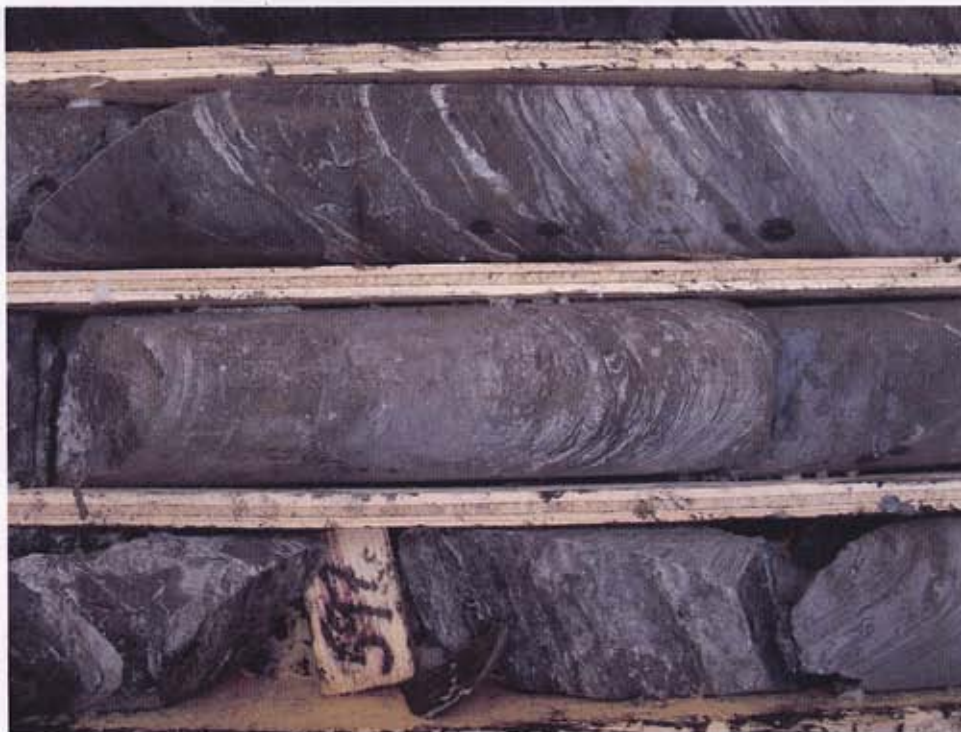
Plate 6. Banded barite-sulphides, mostly pyrite and sphalerite, with minor galena.
