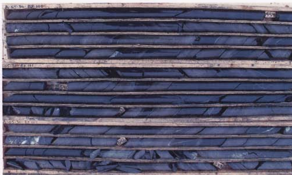
Plate 4. Interbedded black shale and laminated siliceous siltstone- pyrite ± sphalerite.
