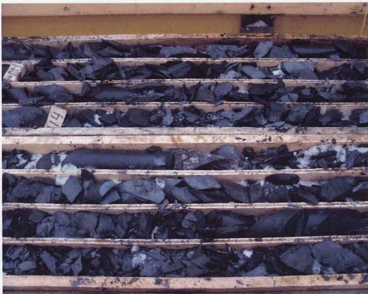
Plate 3. Shattered Gunsteel shale.
