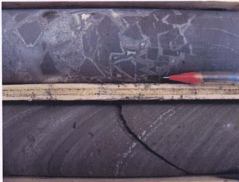
Plate 7. Typical deformation in sulphide beds.
