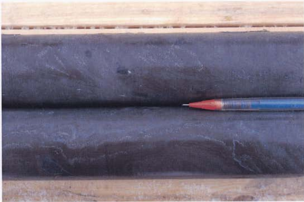
Plate 7. Typical deformation in sulphide beds.
