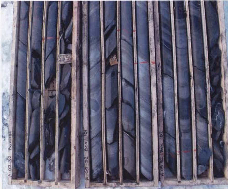
Plate 5. Laminated siltstone-pyrite unit, high in sphalerite. The pale grey bands contain high amounts, up to 40% very fine sphalerite.
