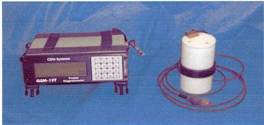
QuickTracker (GSM-19T) console with sensor and cable. Can also be configured with additional sensor for gradiometer(simultaneous) readings.
