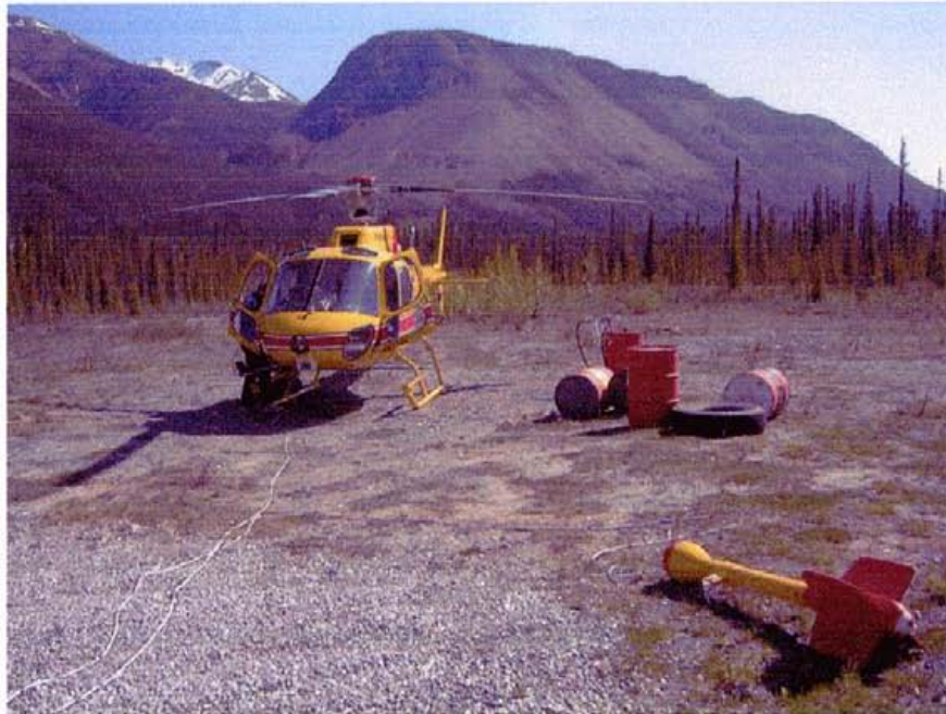
Figure 5: Geometrics G822-A cesium magnetometer mounted in the towed-bird airfoil
