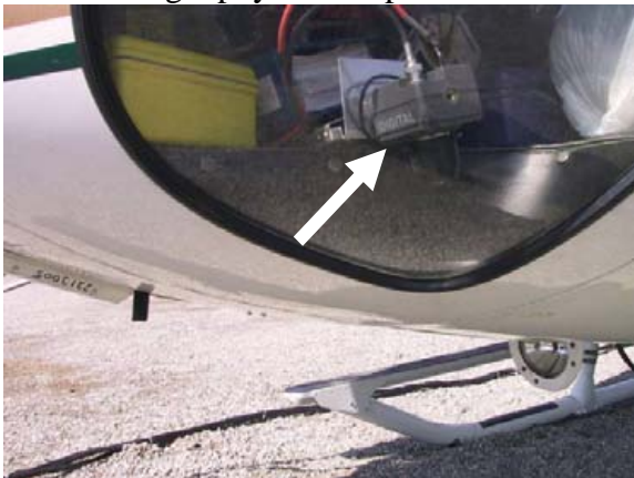
Figure 7. Digital video camera typical mounting location.
