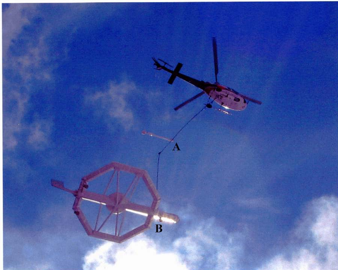
Figure 4. The magnetometer bird (A) and AeroTEM II EM bird (B)
