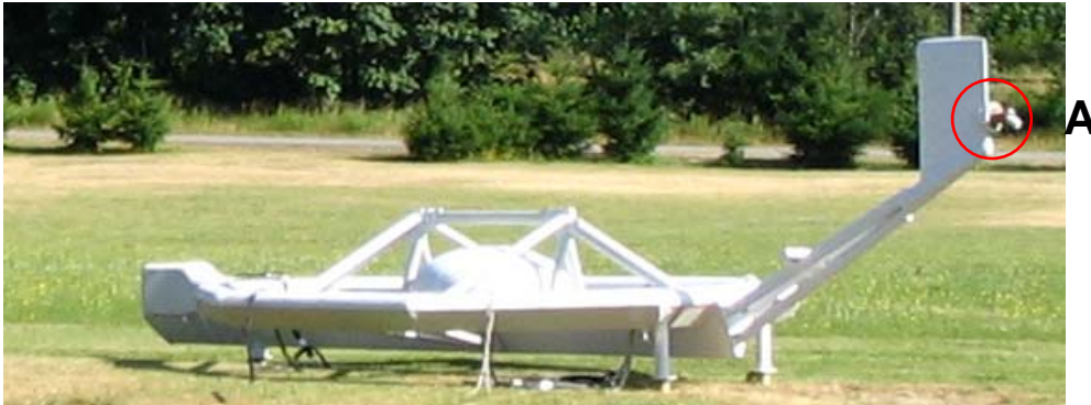
Figure 5. The magnetometer (A) located on the tail of the AeroTEM II EM bird
