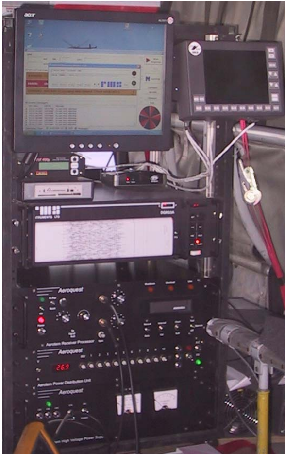
Figure 7. AeroTEM II Instrument Rack. Includes (AeroDAS system and RMS DGR-33 and AeroTEM power supply, data acquisition computer and AG-NAV2 navigation)
