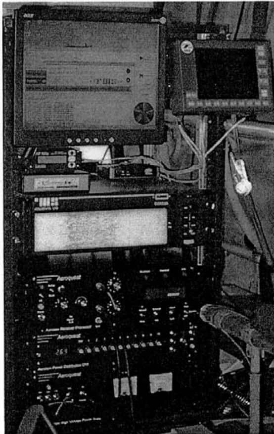
Figure 9. AeroTEM II Instrument Rack. Includes (AeroDAS system and RMS DGR-33 and AeroTEM power supply, data acquisition computer and AG-NAV2 navigation)
