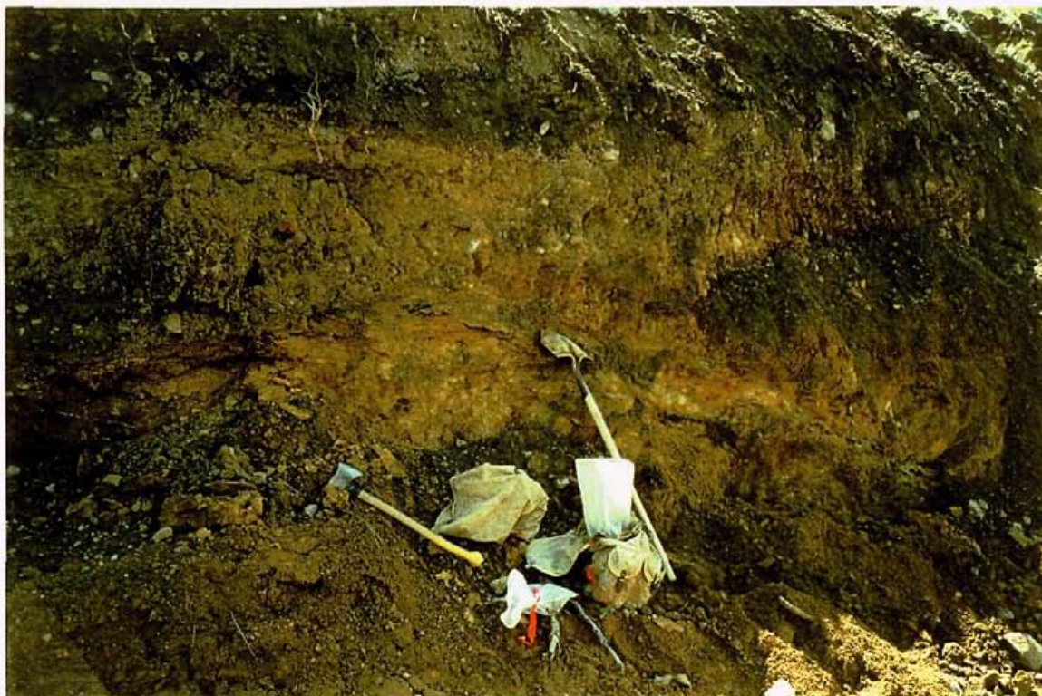
MEGATON: TRENCH NO. 1, SOUTH WALL SHOWING SAPROLITIC GOSSAN ZONE AND FLAT-DIPPING MALACHITE-STAINED QV ZONE ENVELOPED BY INTENSE SERICITE-KAOLIN ALTERATION. SHOVEL POINT AT OVERBURDEN CONTACT
