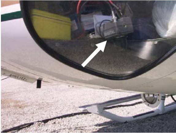
Figure 7. Digital video camera typical mounting location.
