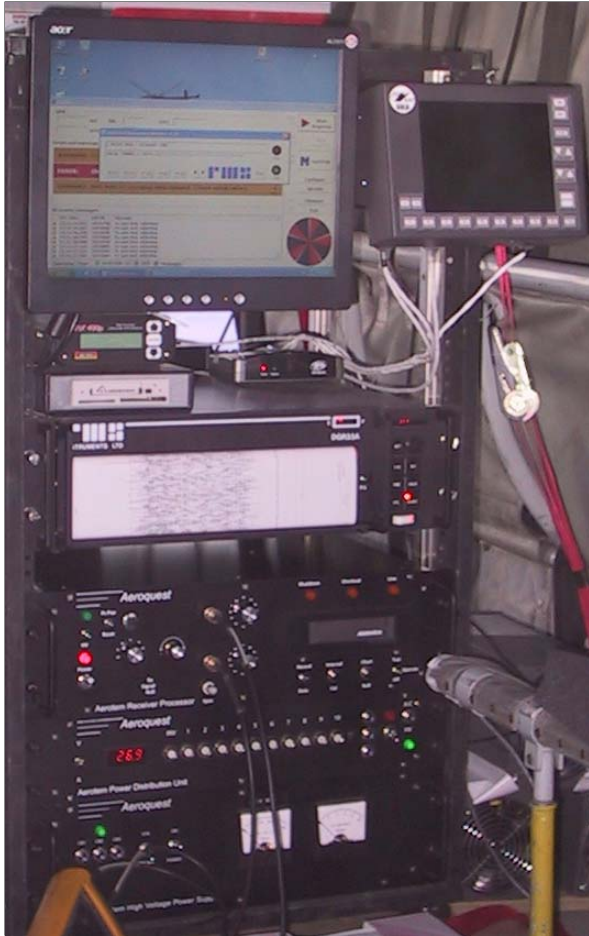
Figure 6. AeroTEM II Instrument Rack. Includes (AeroDAS system and RMS DGR-33 and AeroTEM power supply, data acquisition computer and AG-NAV2 navigation)
