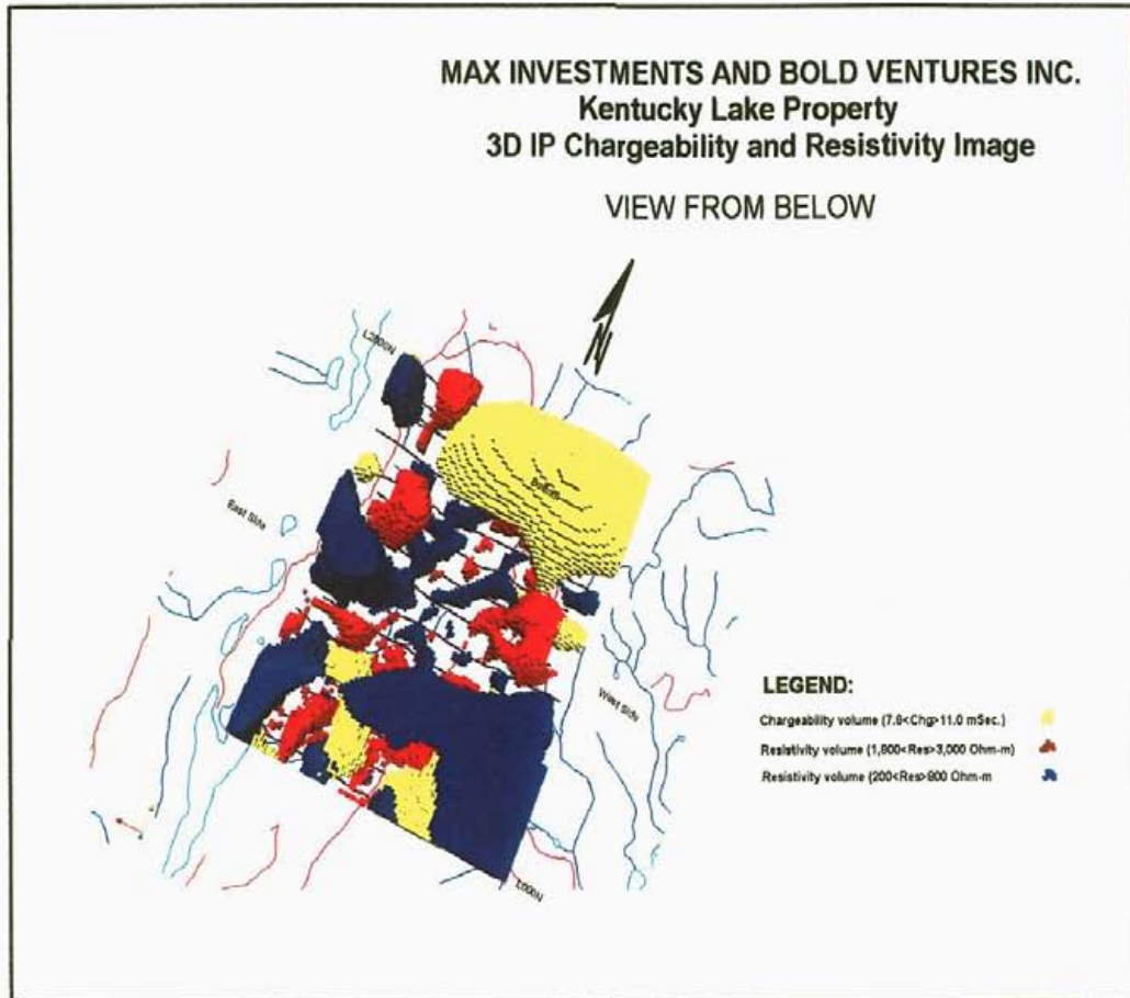
Illustration 6: 3D IP Chargeability and Resistivity Image (viewed from bottom)
