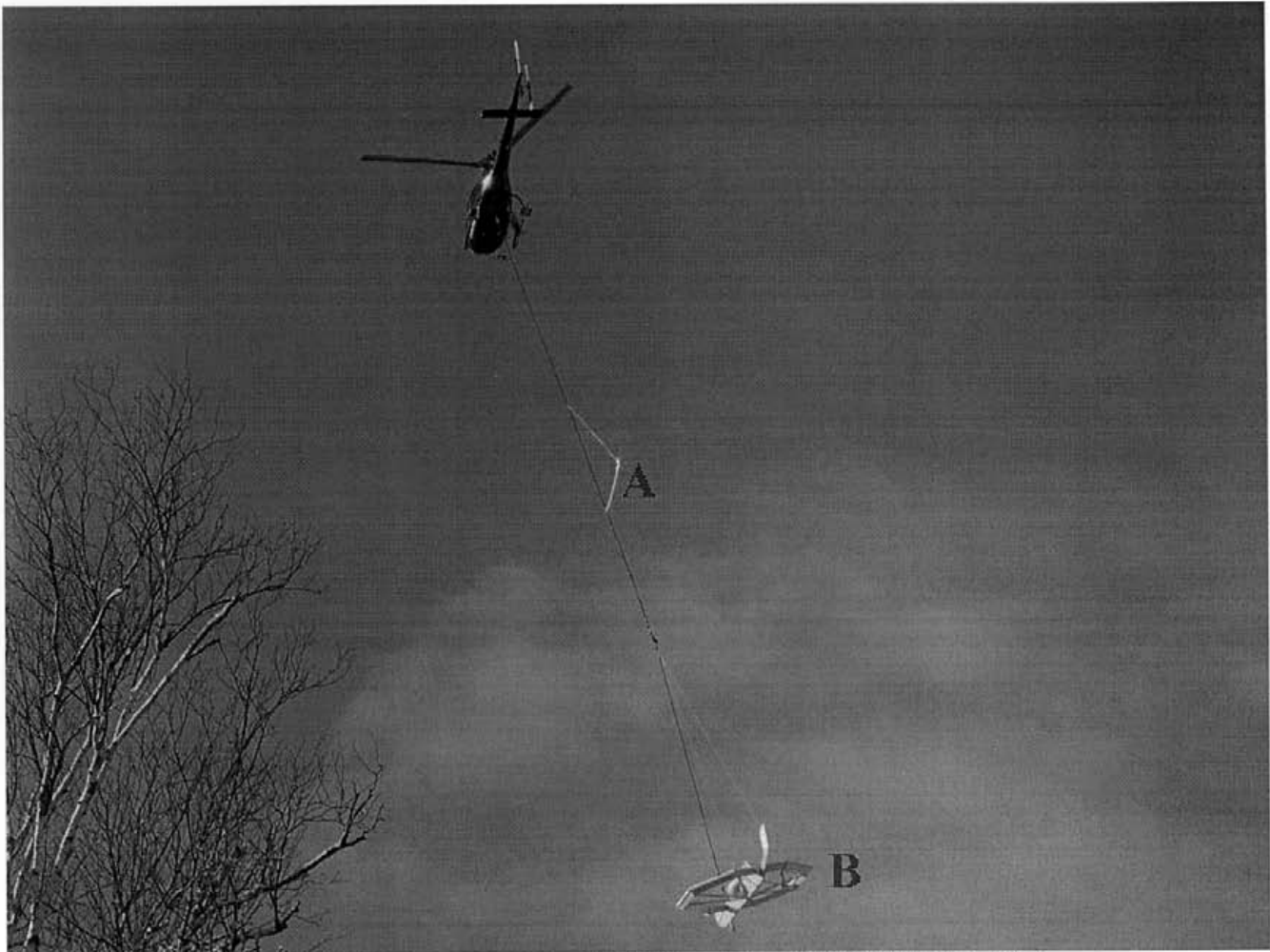
Figure 4. The magnetometer bird (A) and AeroTEM II EM bird (B)
