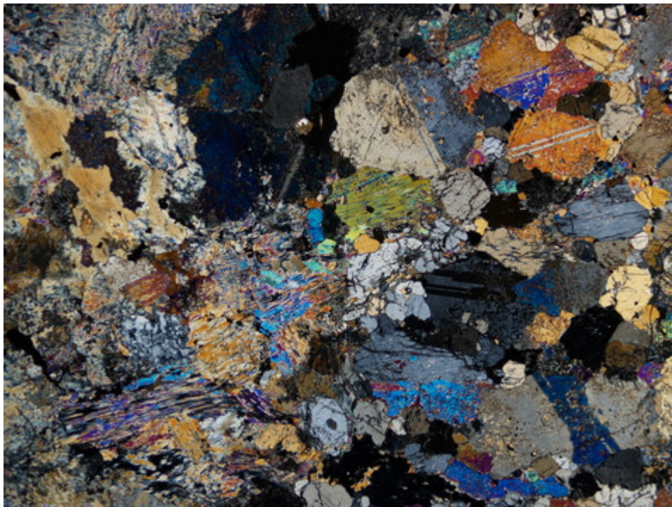
08 - A: A & B) Overview of the sample showing lamellar, locally twinned pyroxenes locally altered by fine foliated actinolite (left side) with interstitial hornblende. A) PPL, B) XPL, FOV = ~ 8.5 mm.
