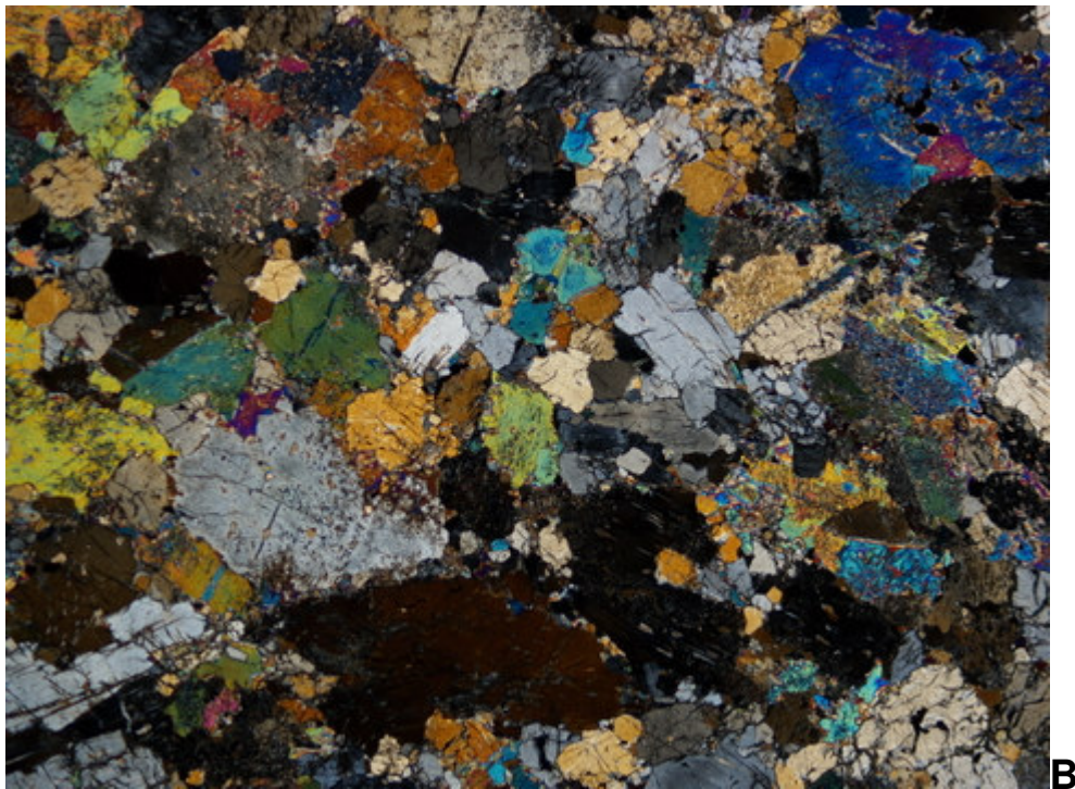
SPX - 02: A & B) Representative view of the sample showing a corroded assemblage of ortho- and clinopyroxene with fine disseminated masses of brown phlogopite..
