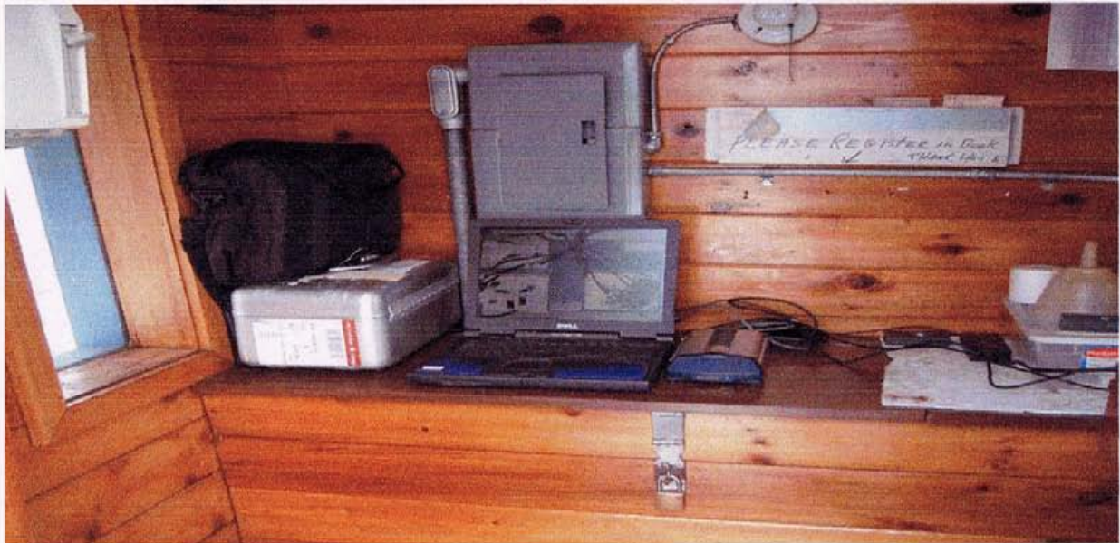
Figure 5: Basestation GPS and magnetometer setup
