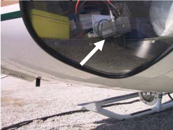
Figure 7. Digital video camera typical mounting location.
