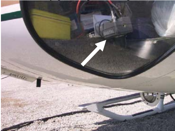
Figure 7. Digital video camera typical mounting location.
