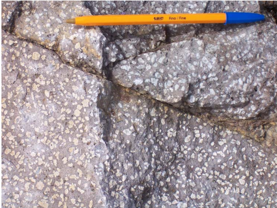
Photo 8: Tertiary feldspar porphyry dyke with fine-grained to aphanitic K-feldspar rich matrix in the western part of map area (stn. TH-25).
