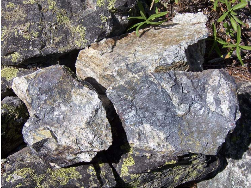
Photo 11: Vein and massive hematite in brecciated Okanagan granitic rocks, east zone (stn. TH-94).
