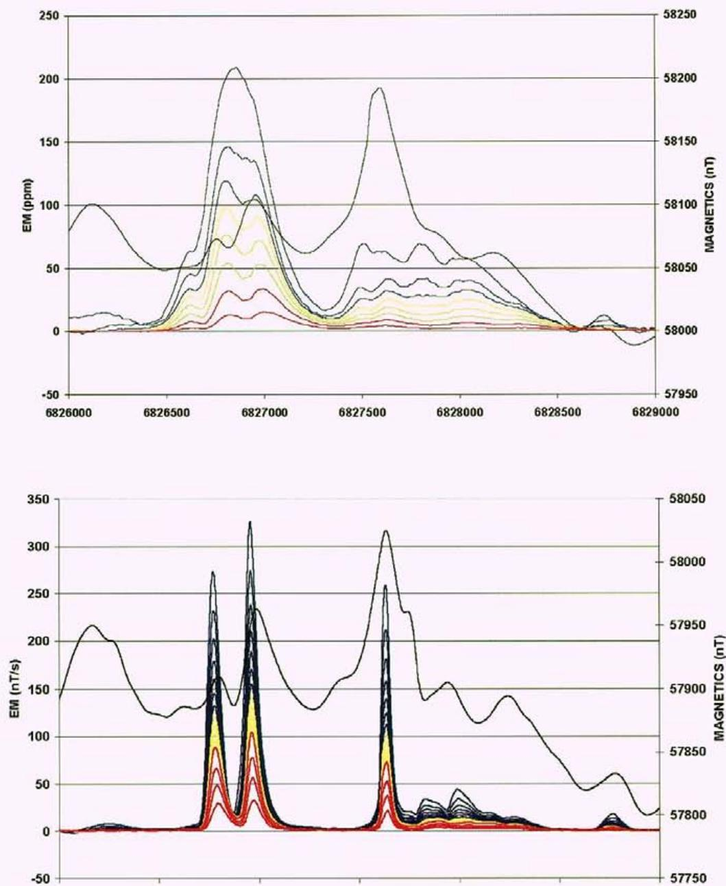
**Figure 2. Fixed-wing (upper) and AeroTEM (lower) comparison over the eastern limit of the Mesamax Deposit, a Ni-Cu-PGE zone located in the Raglan nickel belt and owned by Canadian Royalties. Both systems detected the Deposit further to the west where it is closer to surface.**
