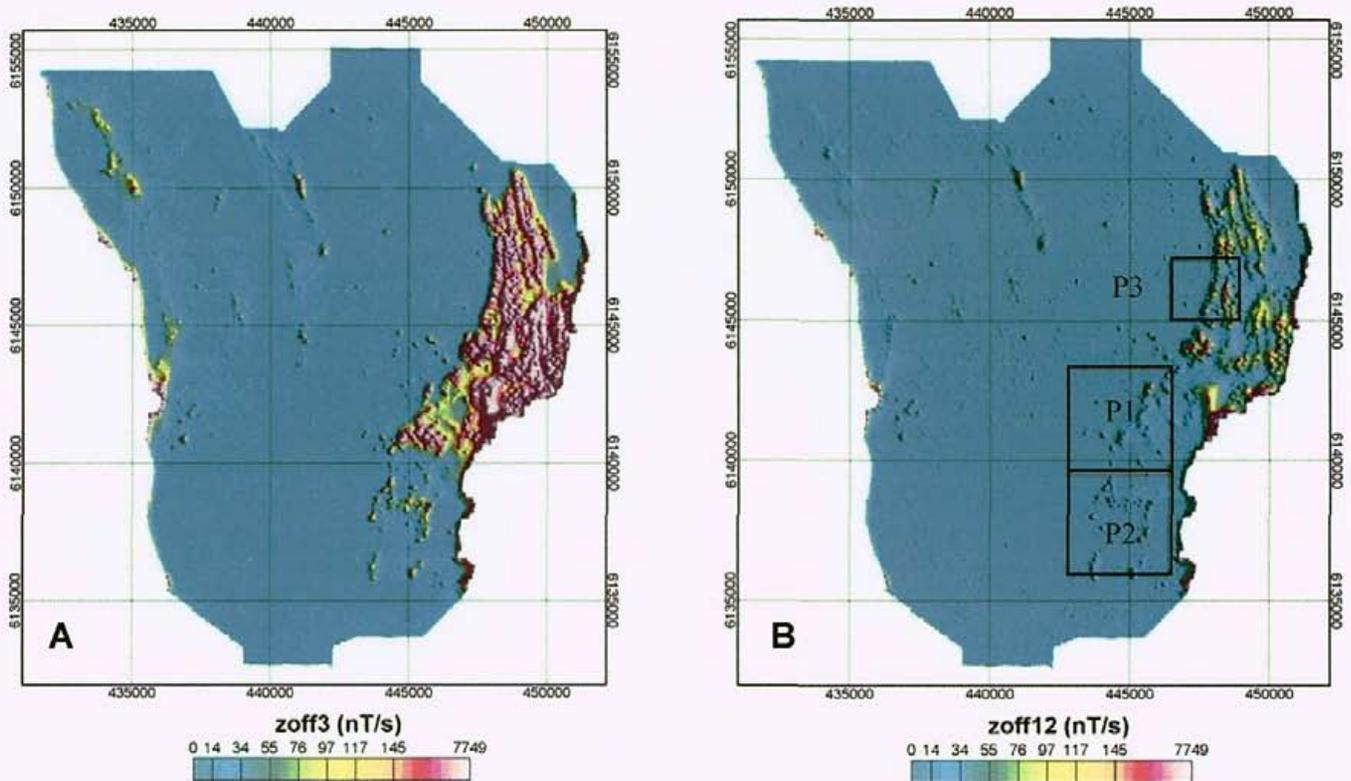
Figure 13. A) Z3 Off-time colour grid B) Z12 Off-time colour grid, highlighting higher conductance sources.
