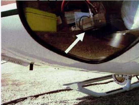
Figure 8. Digital video camera typical mounting location.
