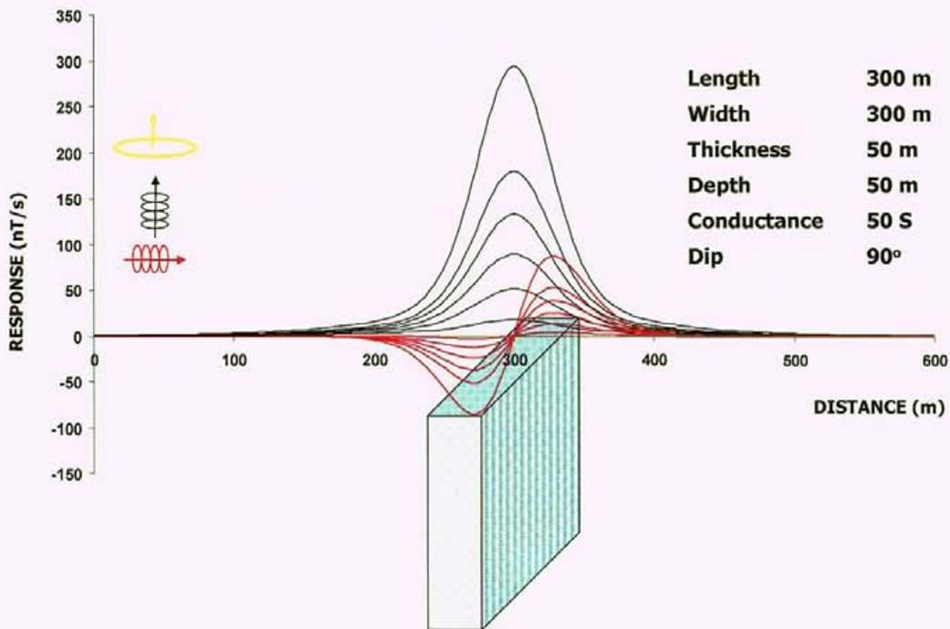
Figure 11. AeroTEM response for a 'thick' vertical conductor.
