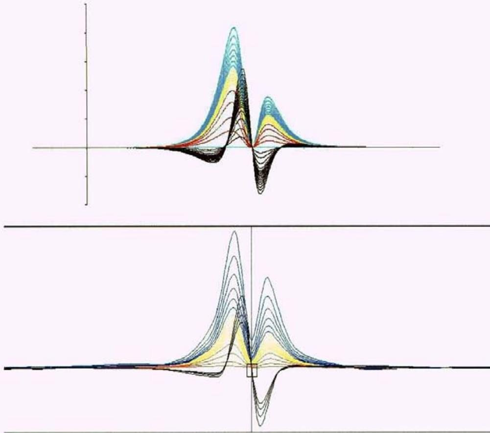
**Figure 5. Measured (lower) and modeled (upper) AeroTEM responses are compared for a thin steeply dipping conductor. The response is characterized by two peaks in the Z-axis coil, and a cross-over in the X-axis coil that is centered between the two Z-axis peaks. The conductor dips toward the higher amplitude Z-axis peak. Using the X-axis cross-over is the only way of differentiating the Z-axis response from being two closely spaced conductors.**
