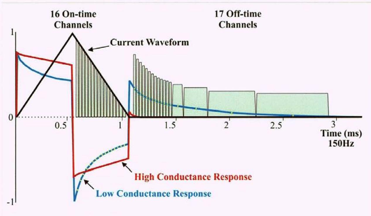
Figure 6. Schematic of Transmitter and Receiver waveforms
