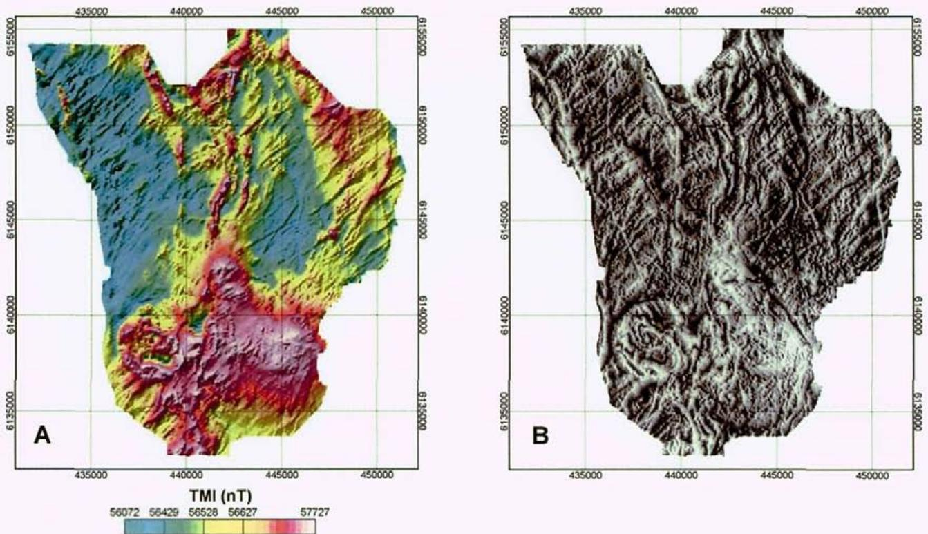
Figure 9. A) Total magnetic intensity map (illumination from the NW). B) TDR Map presented with a grey colour-scale to highlight subtle magnetic lineaments.
