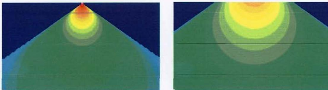
The footprint of AeroTEM at the earth's surface is roughly 50m on either side of transmitter
