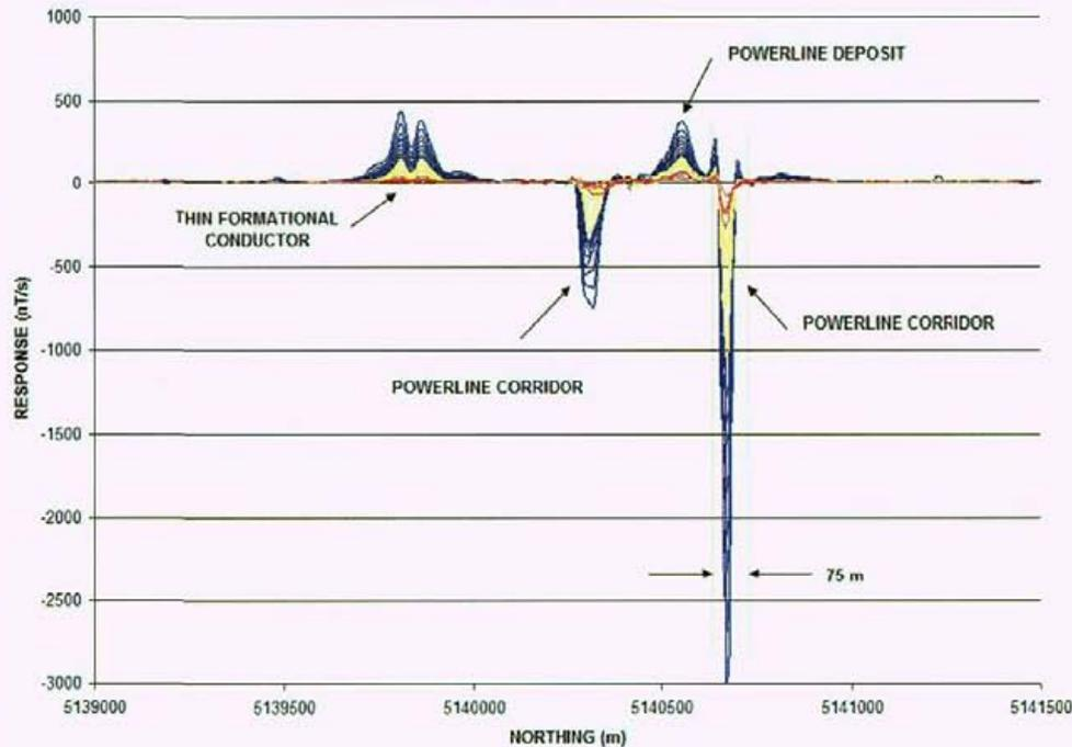
**Figure 3. The Powerline Deposit is located between two major power line corridors, which make EM surveying problematic. Despite the strong response from the power line, the anomaly from the Deposit is clearly detected. Note the thin formational conductor located to the south. The only way to distinguish this response from that of two closely spaced conductors is by interpreting the X-axis coil response.**
