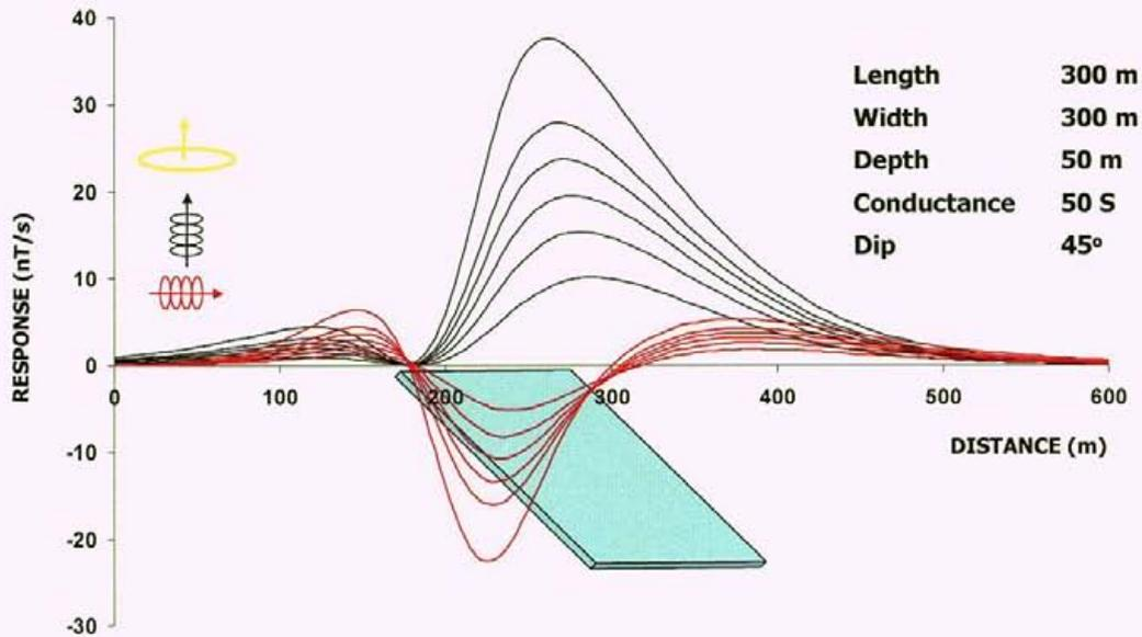
Figure 12. AeroTEM response over a 'thick' dipping conductor.
