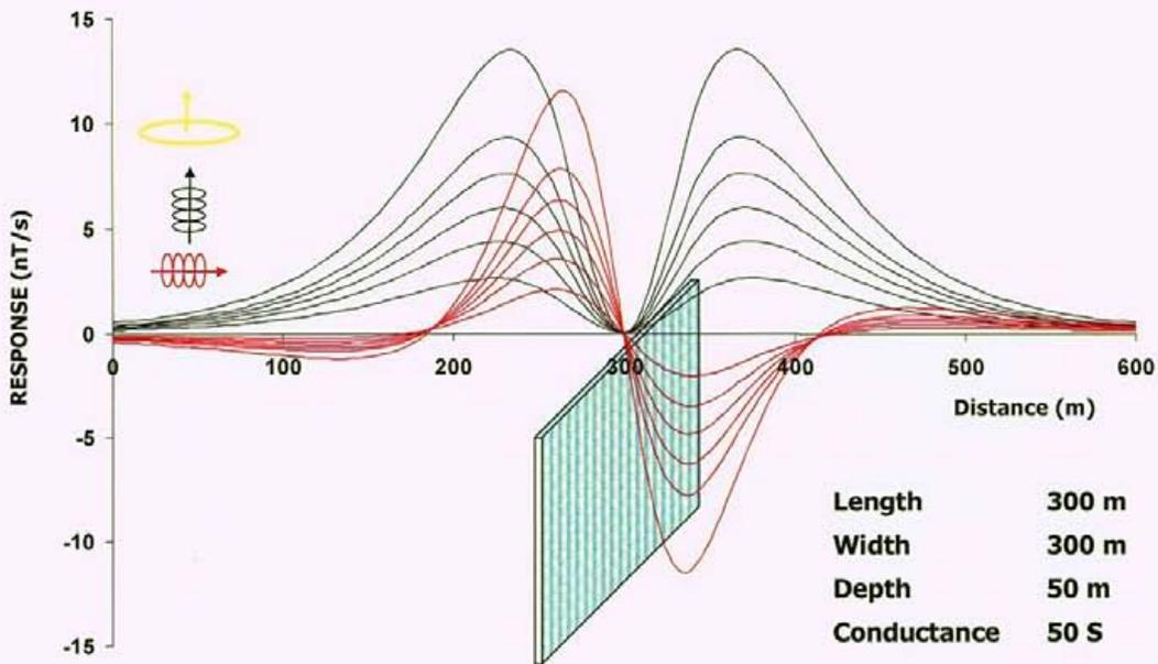
Figure 10. AeroTEM response to a 'thin' vertical conductor.
