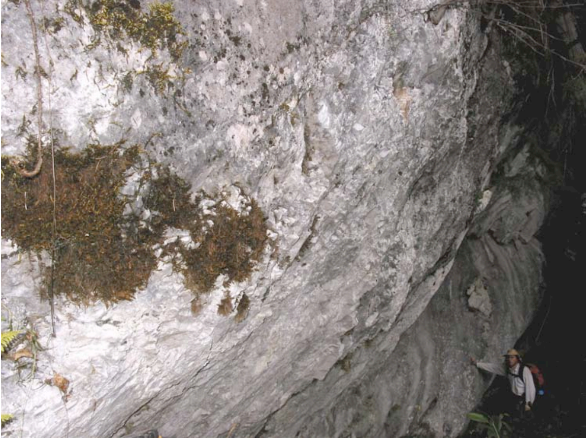
Fig. 4: Photo of part of the marble cliff, proposed quarry test area of Map 6, showing white marble coated with dark lichen. Note arcuate slip fracture directly above Anatoliy.
