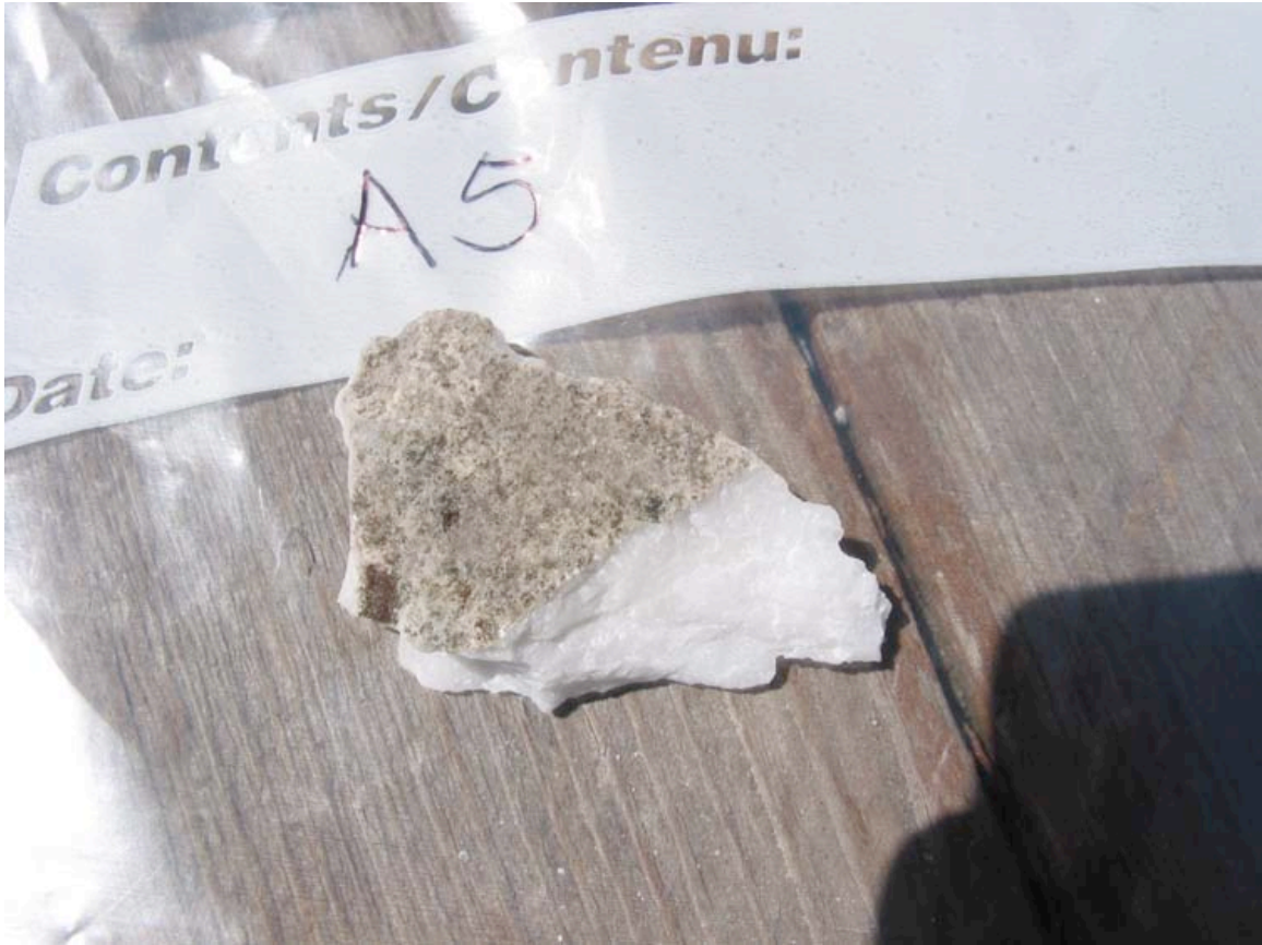
Fig. 6: Chip of microcrystalline marble showing lichen rind collected from the marble cliff face of figure 4.
