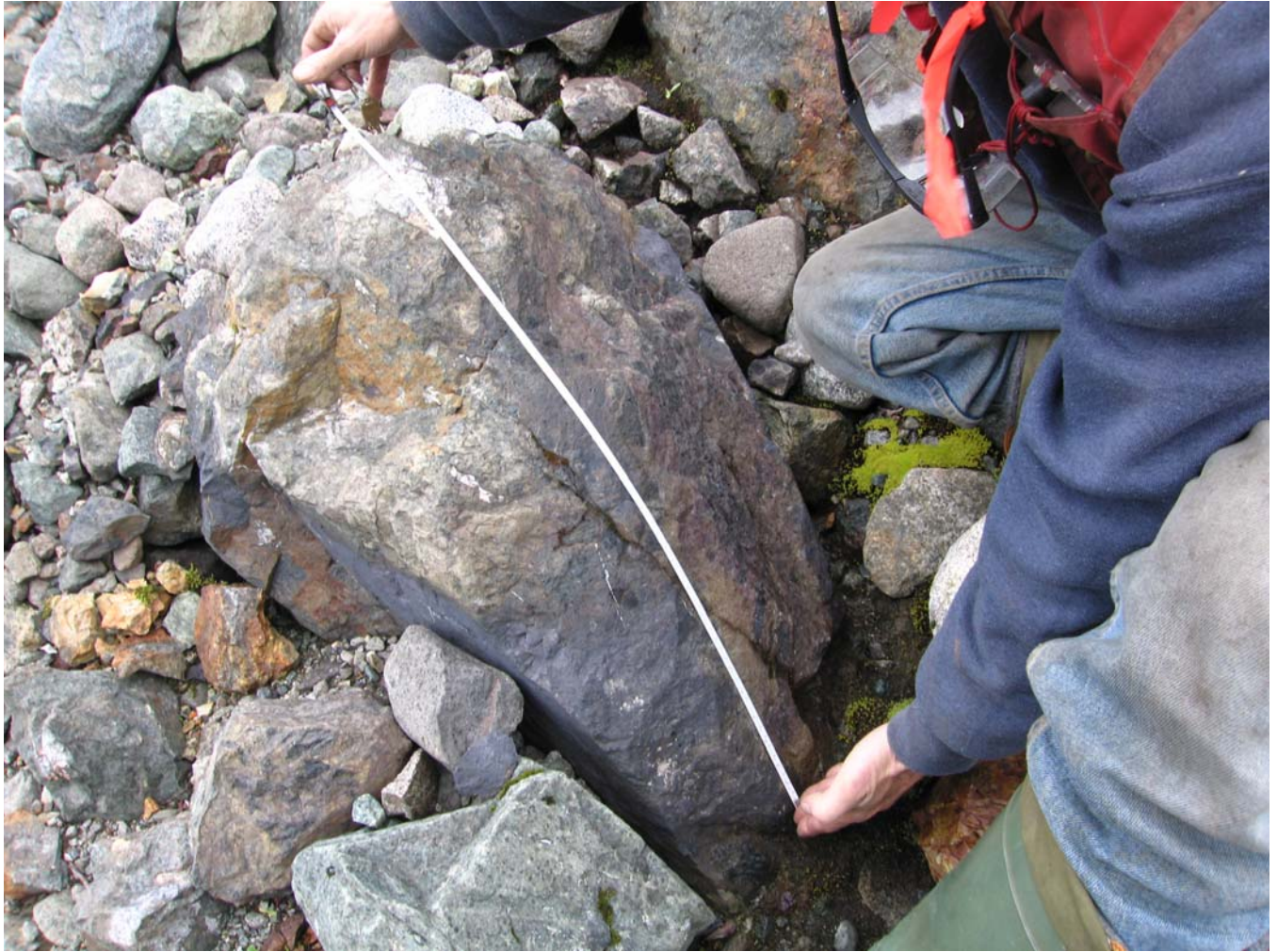
Photo 10. Zone A: Typical boulder of massive sulphides, which give assay returns up to 62.7 g/t Au and 79.5 g/t Ag. Note deceptive colour of boulder. Although massive sulphides its colour is much the same as adjacent barren rocks. Details of assays from boulders are given below.
