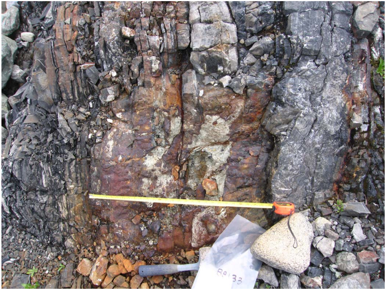
Photo 7. Zone B: Discontinuous and in echelon lenses of stratiform sulphides, up to five metres long, 60 cm thick, spread over 107 metres in vertically dipping black argillaceous shales, striking 130 deg/88deg N. Year 2006 chip sample assay returns 60 cm lengths giving up to 6.93 g/t Au, 36.2 g/t Ag, 3.2% Pb, 16.4% Zn. Details of chip sample returns provided in table below.
