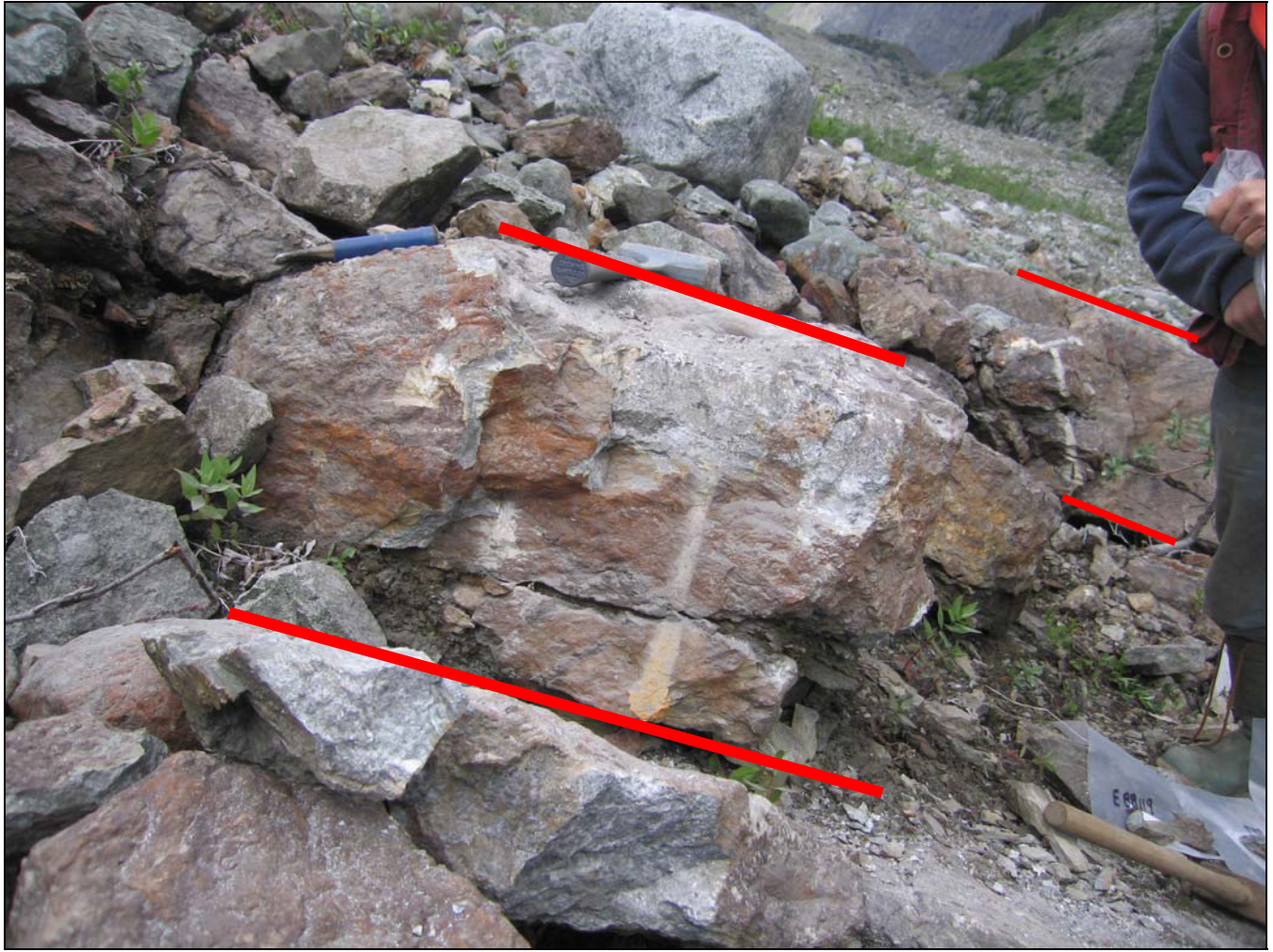
Photo 5. Zone C: Looking West. Contact zone looking down strike of massive sulphide lens 1.20 metres thick. Host rock is altered Stikine Assemblage sedimentary rock, outboard to hydrothermal breccia, not shown. Note glacial gravel and boulder debris upper right, typically covering 85%-90% of the sulphide mineralized zone. A drill hole located within hydrothermal breccia left (not shown) would have drilled down dip and underneath this massive sulphide lens. Table below shows results of 5 chip samples across this lens section at 1 metre intervals, (total length of lens sampled = 5 metres).
