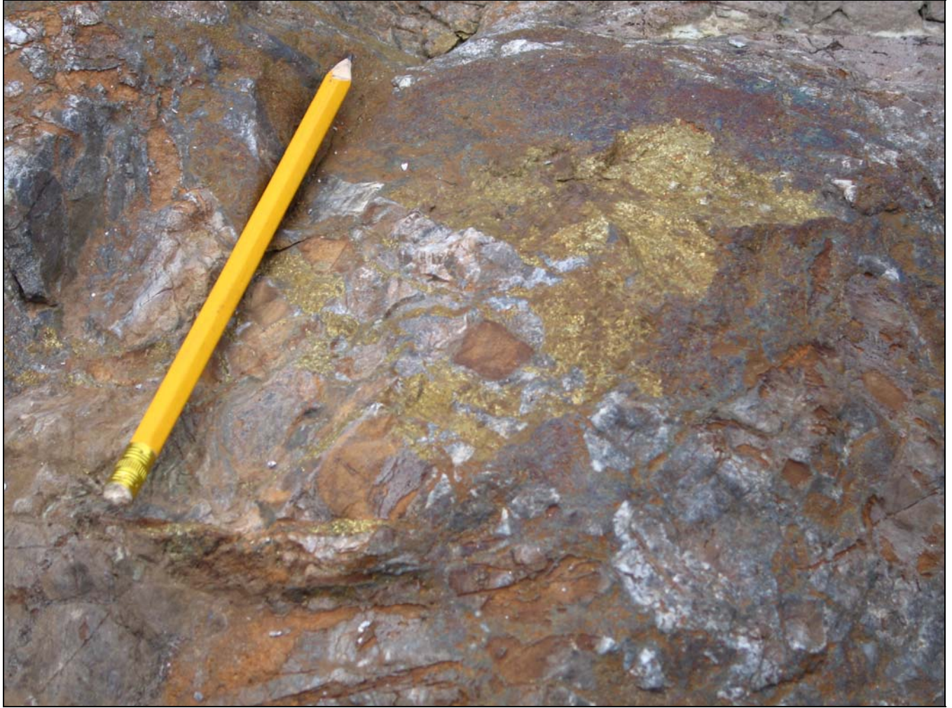
Photo 4. Zone C: Hydrothermal breccia contact zone showing massive sulphides lens 10 cm thick, after weathered surface chipped off with chisel. 2006 Assay returns up to 9.26 g/t Au, 202 g/t Ag, 4.14 % Cu, 3.27 % Pb, 15.5% Zn
