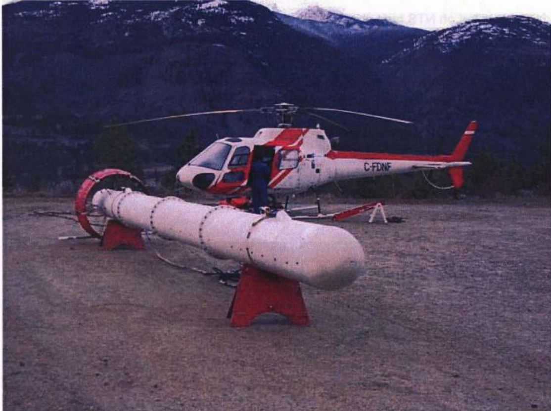
Figure 1: Fugro Airborne Surveys DIGHEM EM bird with AS350-B2
