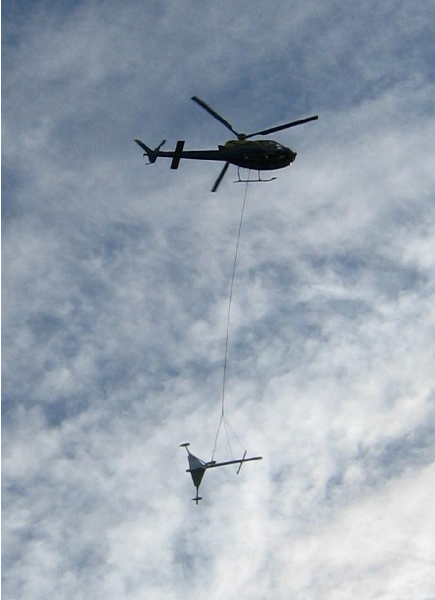
Figure 5. HELI-MAG Magnetic Gradiometer Bird and helicopter on survey.
