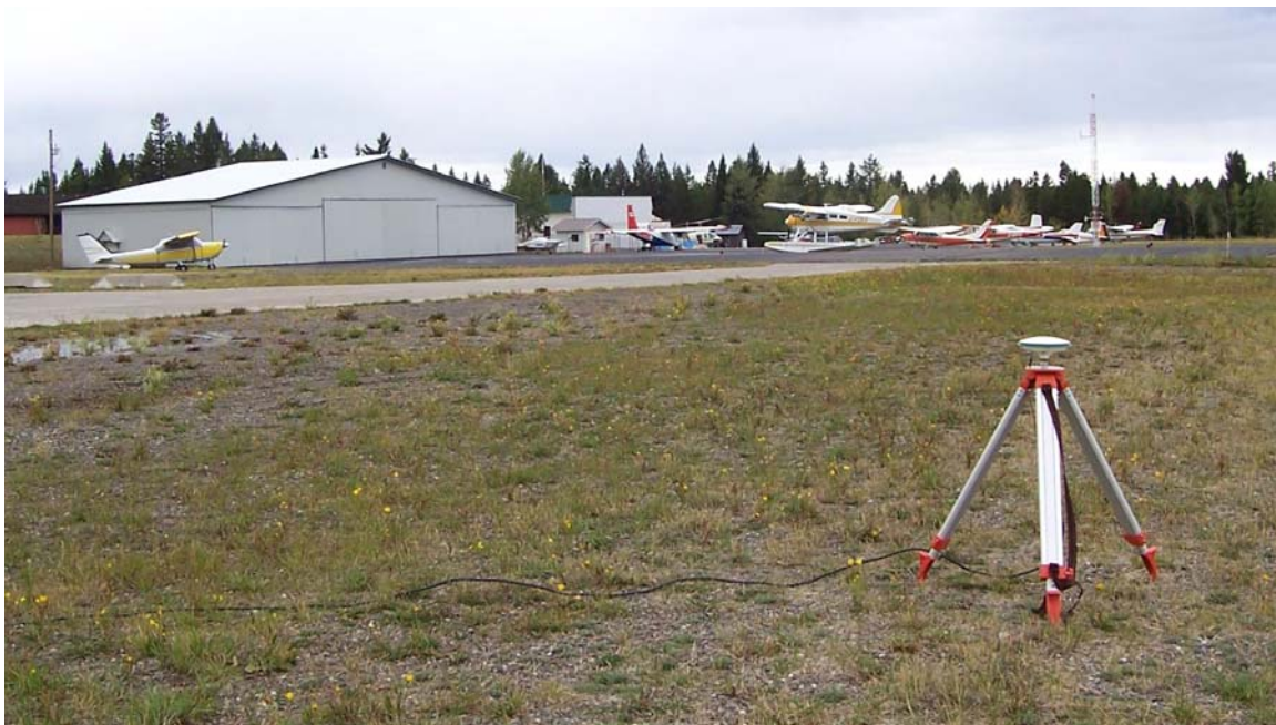
Picture 5: GPS Antenna of the Base Station at 108 Mile Ranch Airport
