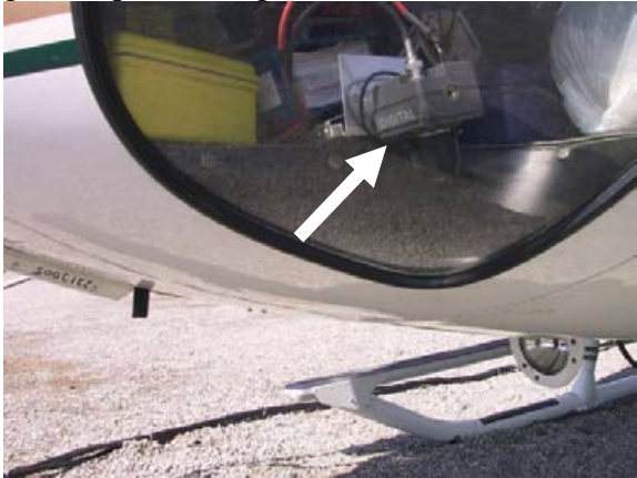
Figure 7. Digital video camera typical mounting location.
