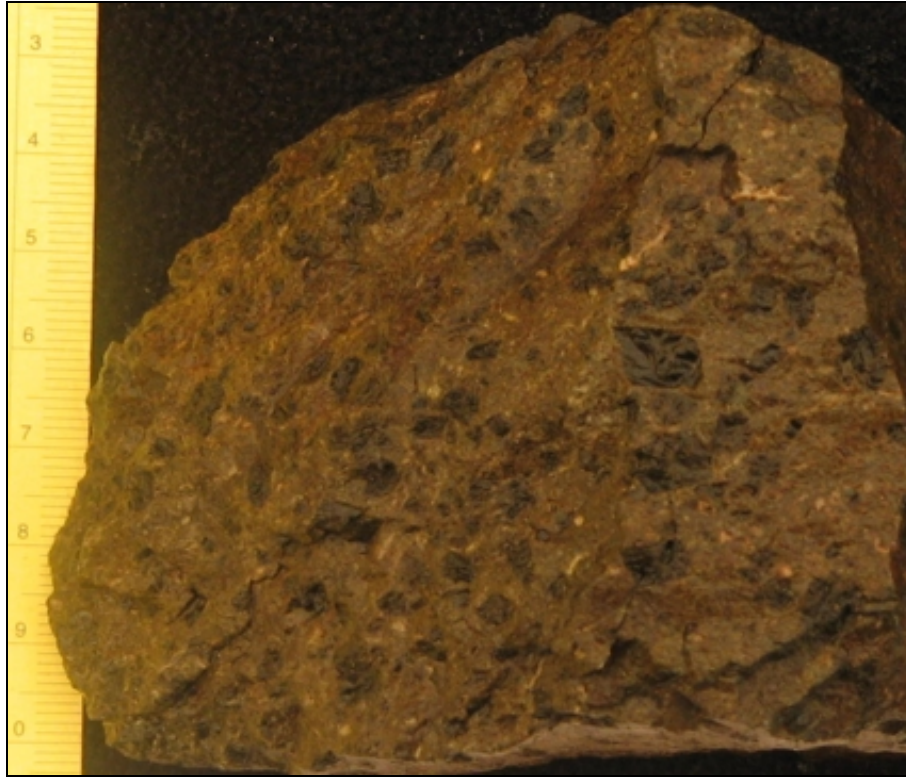
Photo 3.2. Basaltic volcanic of unit 2, with (A) quartz and calcite-filled amygdules, and (B) megacrystic augite phenocrysts. The scale is in centimeters for both images.
