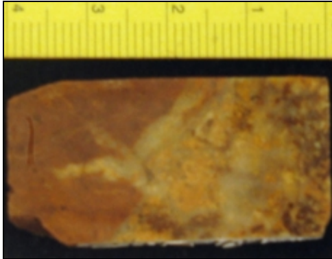
Photo 20: SJ06-104. Iron carbonate and quartz alteration have entirely altered the protolith. The scale is in centimeters.
