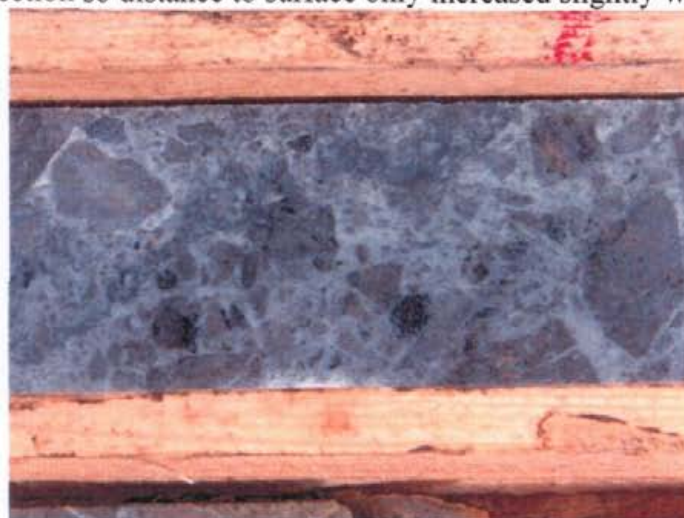
Figure 3.1 Carbonate healed tectonic breccia in drill-core from CMP207-29. Interval is 61' long.
