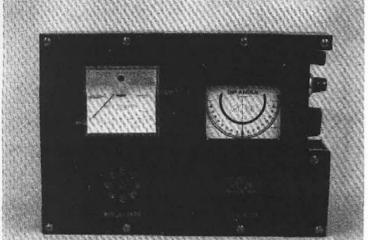
An EM receiver measuring the FIELD STRENGTH, DIP ANGLE and QUADRATURE components of the VLF communications stations.
