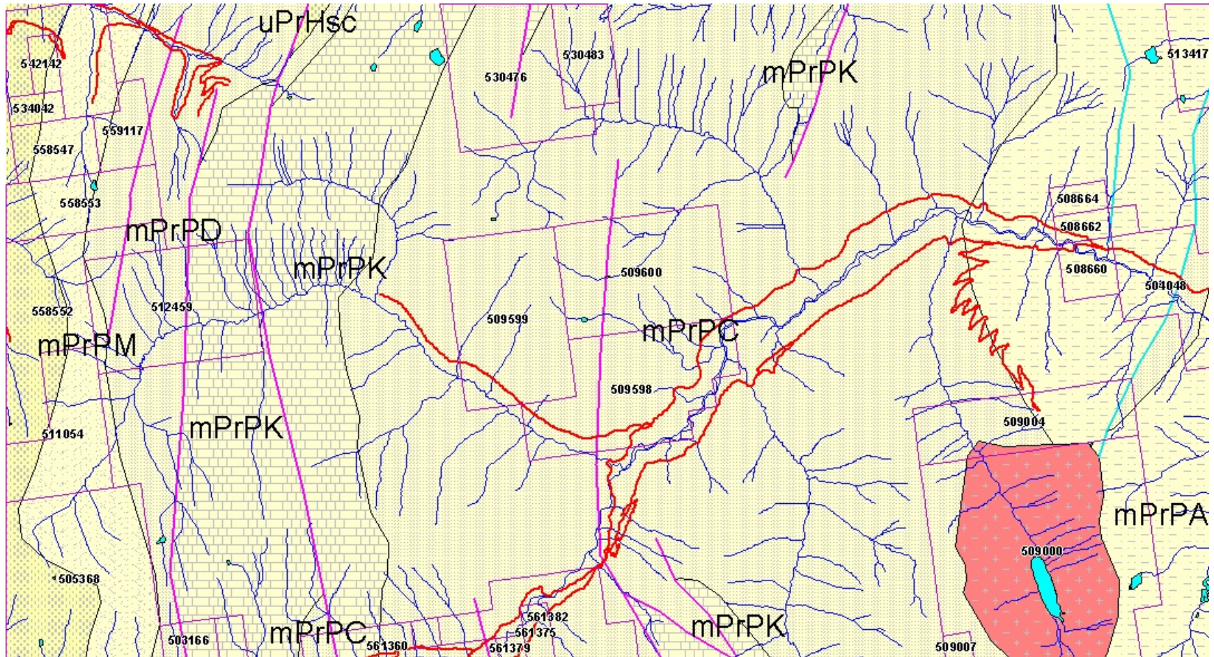
Figure 4: Regional Geology map for Baribeau property. Property underlain by middle Proterozoic Creston Formation (mPrPC). Fault duplication evident through centre of property. Note Hall Lake Stock at lower right (Approximate scale 1: 75,000). Map taken from The MapPlace.
