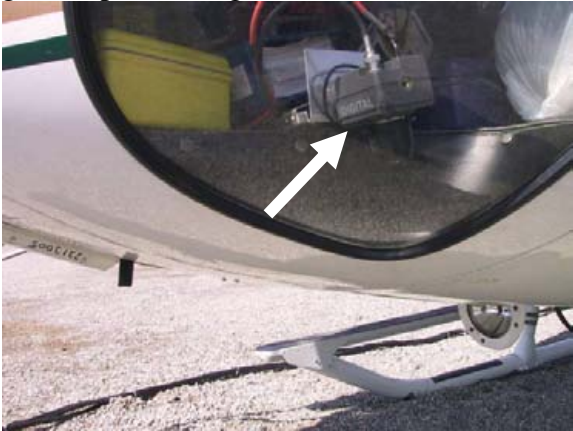
Figure 7. Digital video camera typical mounting location.
