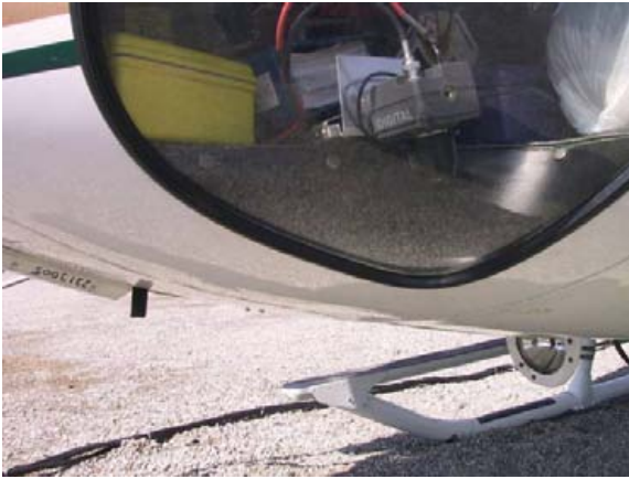
Figure 8. Digital video camera typical mounting location.
