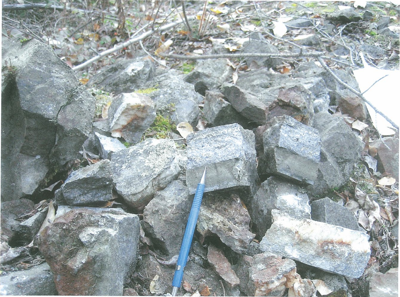
Photograph #2: Richly mineralized spoils dump near JWR shaft and trench. Pencil points to mineral vein fragment; note vein width on spoil samples to be 8 cms. Other mineralized fragments present in photograph, grey colour, associated with white calcite-quartz.
