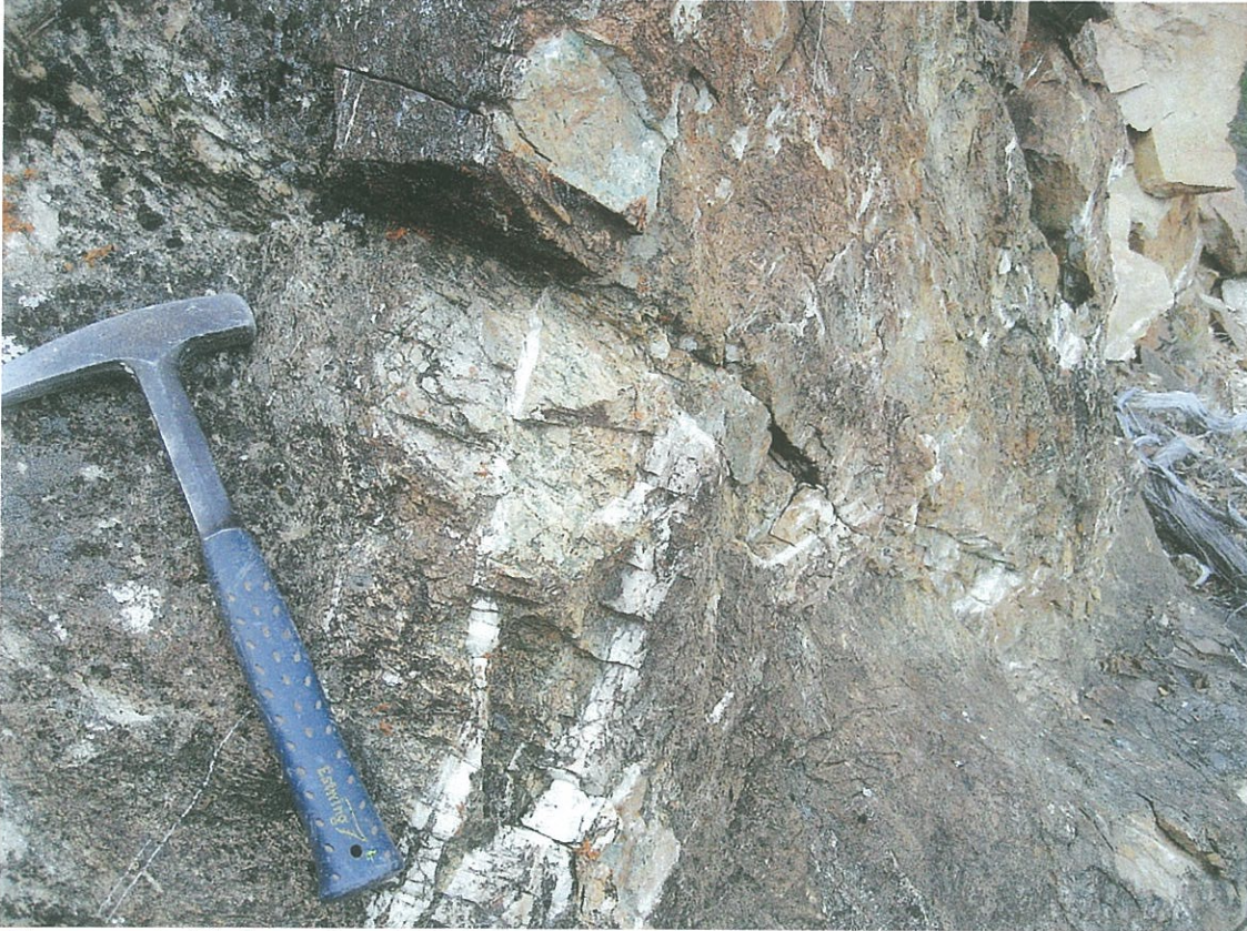
Photograph #4: Location 662948: quartz veinlets in carbonaceous ultramafics. Note green fuchsite above geological pick.
