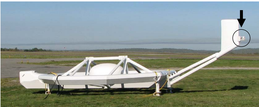
Figure 5. AeroTEM II EM bird. Arrow indicates the location of the second cesium magnetometer sensor.
