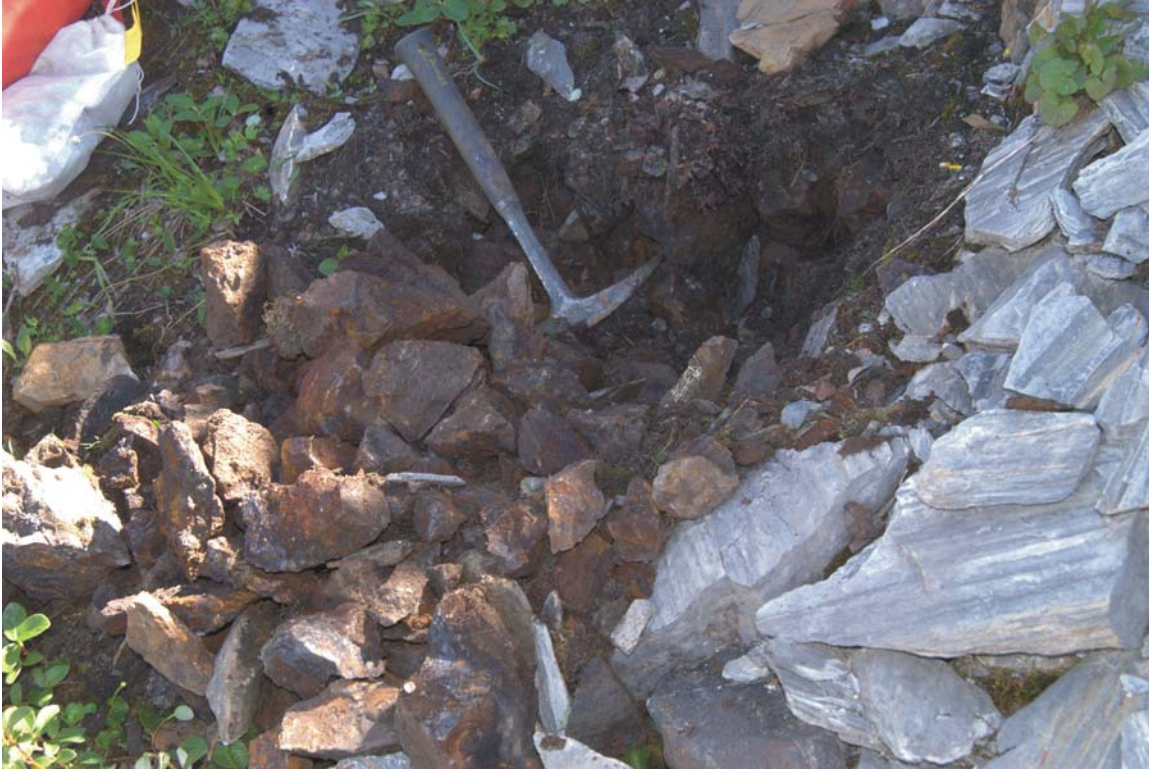
Figure 9: Gossan showing (along strike and north of the “peak 2179” showing). Zone is at least 10 m long and 1 to 2 m wide (ref. map in pocket). It is hosted by grey-banded marble.
