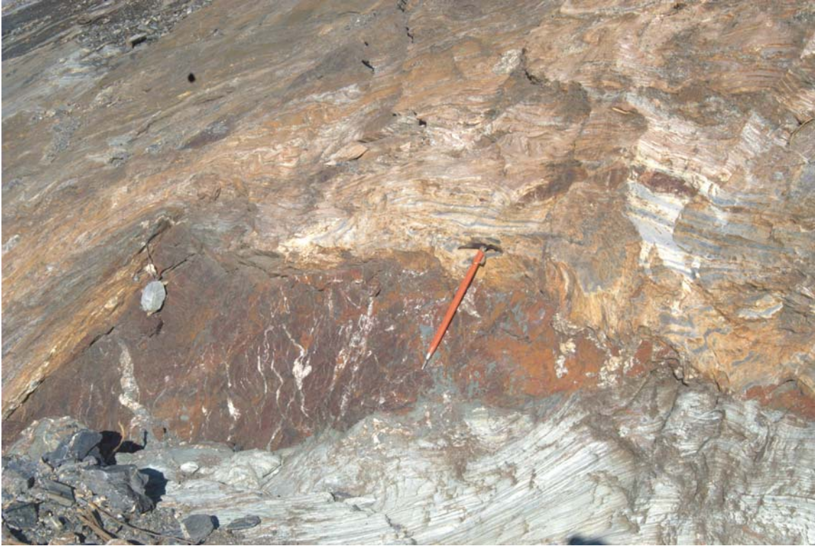
Figure 8: Lens of rusty-brown siliceous marble, bounded by green phyllite (below) and iron-rich marble (above), illustrating the influence of competency on structural style. The less competent phyllite and marble have flowed along fractures into the brittle siliceous marble. Secondary quartz, calcite and sulphide minerals form fracture fillings. Openings along fractures in brittle rocks are ideal sites for deposition of remobilized sulphide minerals.
