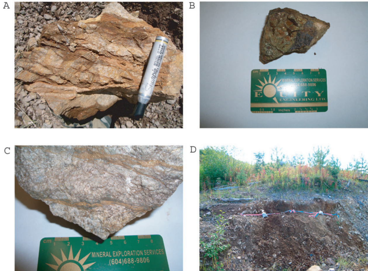
Figure 4: a) Photograph of granodiorite at the Copper Starr showing. b) Photograph of rock from Copper Starr showing with chalcopyrite and pyrite mineralization in ankarite, potassic altered granodiorite. c) Photograph of rock from Copper Starr showing siderite veinlet with dusty chalcopyrite envelope in weakly potassic altered granodiorite. d) Photograph of two 2 m long chip samples over the Copper Starr showing.
