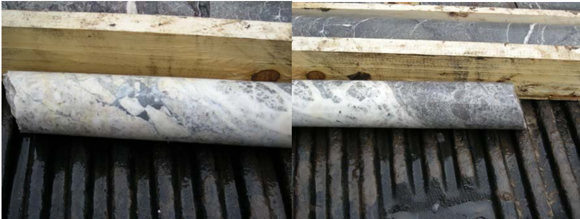
Figure 6: Left, (52.0 –52.37m) jig-saw fit of carbonate clasts in carbonate/silica matrix. Right, (52.37-52.71m) contact of carbonate and silica matrix of zone, 52° (Segment 3).
