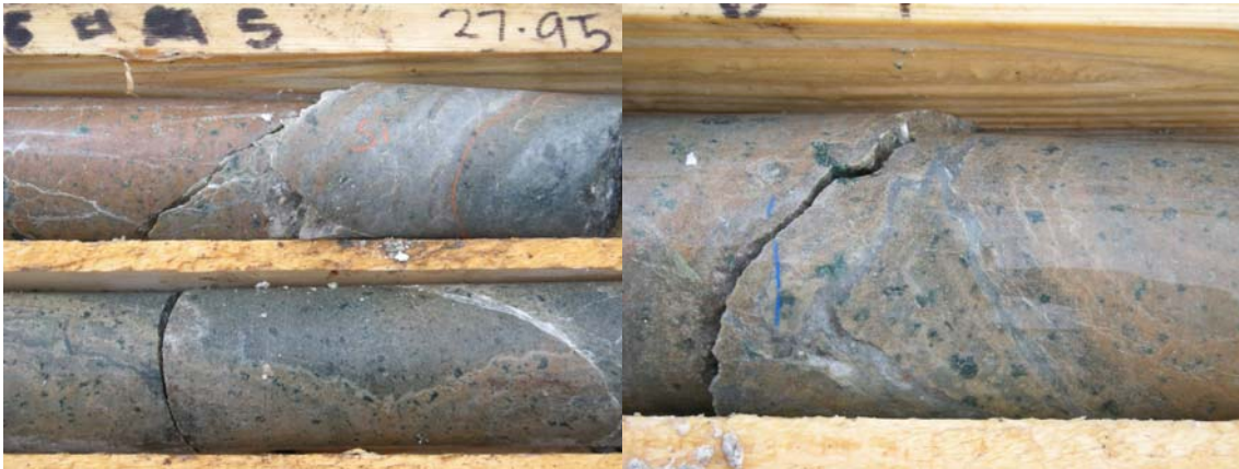
Figure 8: (Left) Silica veining in pink-orange, carbonate altered andesite (28.18–28.41m). (Right) Meandering silica vein in pink-orange, carbonate altered andesite (29.00–29.12m).
