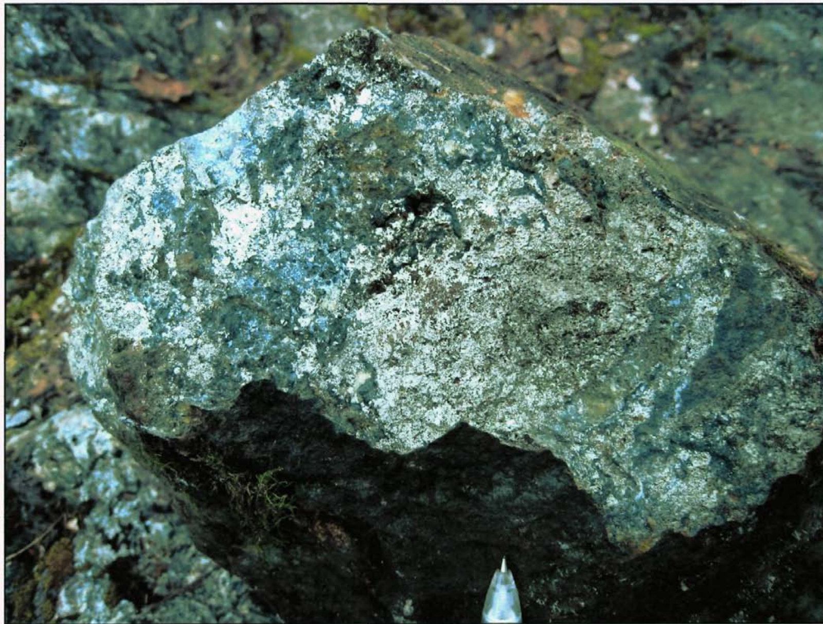
PHOTO 4N SEMI MASSIVE SULFIDE (PY, CPY) BOULDER , SOUTH EXTENSION OF D ZONE SAMPLE 712154: 5.89 g Au/t, 6.1% Cu
