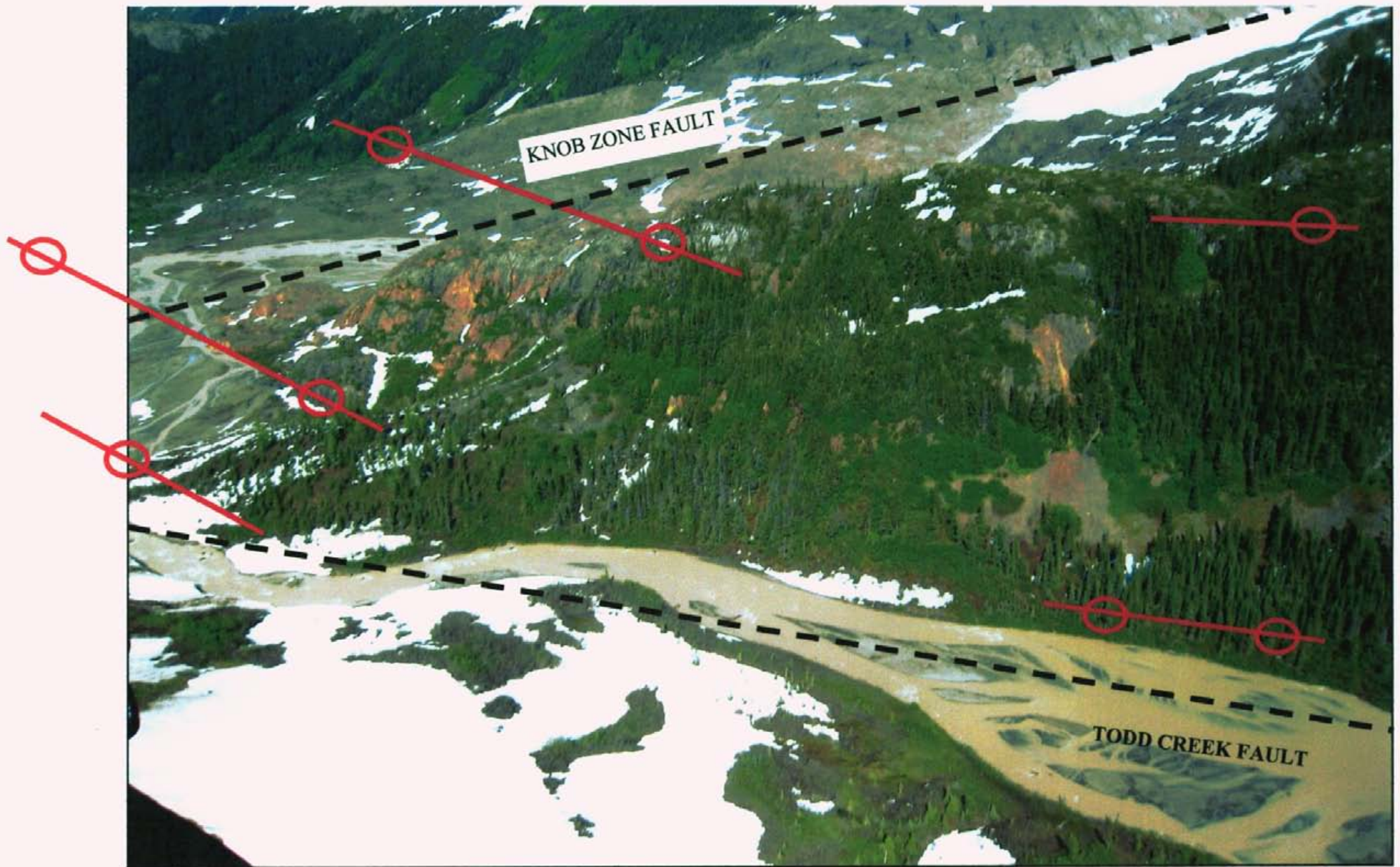
PHOTO 3 KNOB ZONE , LOOKING NE SULFIDE MATRIX BRECCIA "MILL ROCK" AND FELDSPAR PORPHYRY INTRUSIVE WITH AIRBORNE EM ANOMALIES
