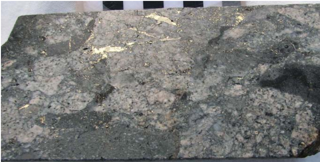
Fig 10-2-8: 06CF287-19.3 m INBX, Intrusive Breccia (polished surface). Closely packed clasts of predominantly granodiorite and minor feldspar porphyry, within a dark grey, fine grained, igneous, felsic matrix. Accessory infilling by chalcopyrite and pyrite as 1 cm stringers and disseminations.
