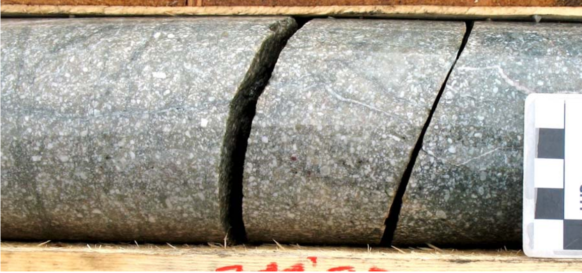
Fig 10-2-5: 06CF284-242.80 m. PPFQ. Feldspar Quartz Porphyry. Strongly feldspar phytic, medium grained, felsic intrusive. Euhedral and subhedral plagioclase phenocrysts in variously textured, fine grained, igneous groundmass with weak potassic alteration.
