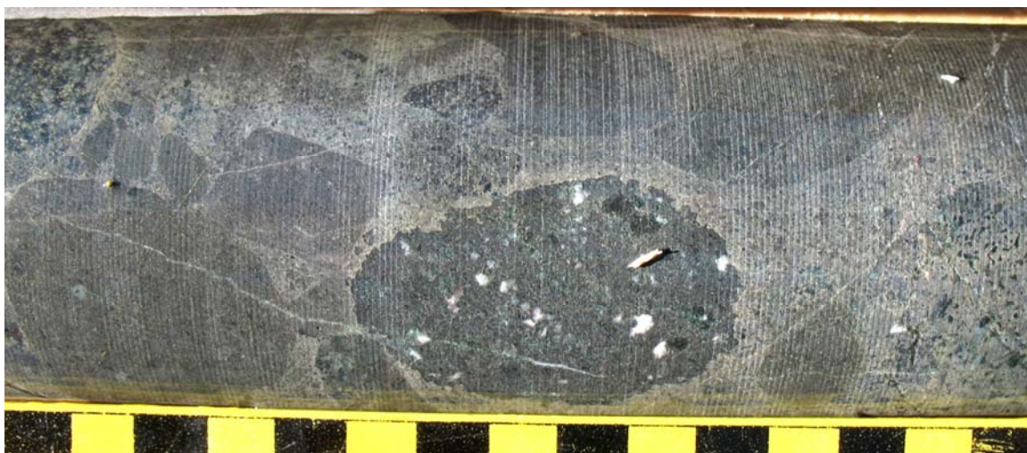
Fig 10-2-12: 06CF273-235.15 m. ANBX. Andesite Lapilli Breccia. Heterolithic volcanic breccia with mm to >10 cm size, rounded and angular clasts in chlorite dominated, 30–50 % matrix.
