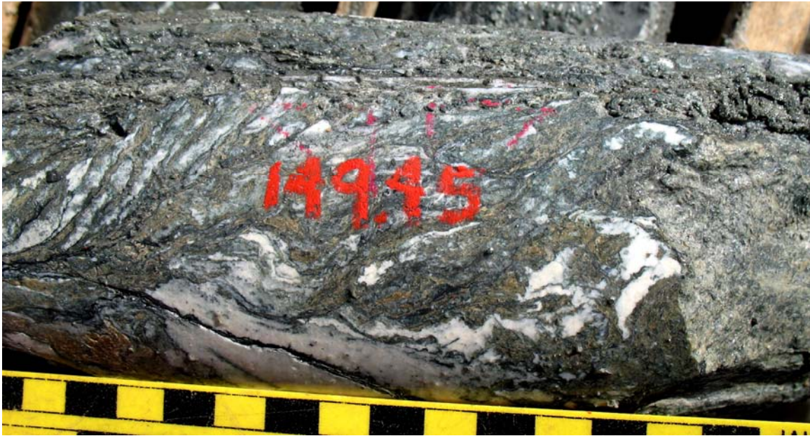
Fig 10-2-20: 06CF268-149.45 m. FAUL/SHER, Faults, Shearing. Mylonitic shearing of phyllically altered andesite, with closely spaced, oriented, parallel carbonate veins.
