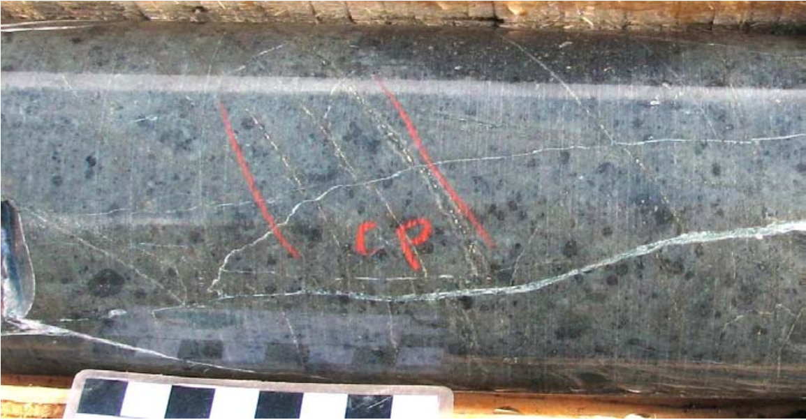
Fig 10-2-17: 06CF258-106.7 m. ANAP, Feldspar-Augite-Phyric Andesite. 10 – 30 % light grey feldspar-phenocrysts and 5% dark green-grey, altered augite phenocrysts within a fine grained igneous groundmass. Note: accessory chalcopyrite is in <1mm wide, sub-parallel stringers.
