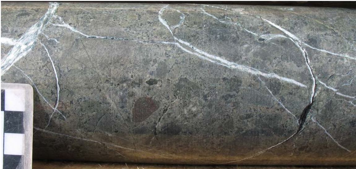
Fig 10-2-13: 06CF256-277.3 m. ANLP, Andesite Lapilli Tuff. Heterolithic, subrounded, mm-2cm andesitic clasts within a fine grained, fragmental crystal tuff matrix, with minor carbonate veins.
