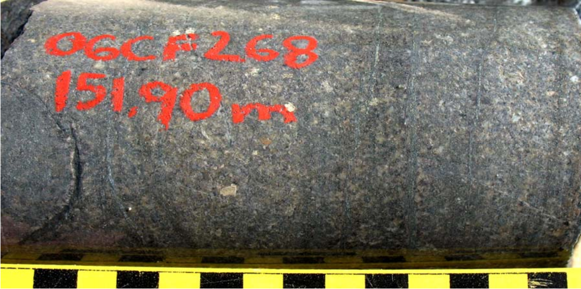
Fig 10-2-6: 06CF268-151.9 m. DIOR, Diorite. This sample is intermediate in composition, equigranular, medium grained and is made up of anhedral to subhedral plagioclase and ~20 % interstitial chlorite and iron magnesium minerals.
