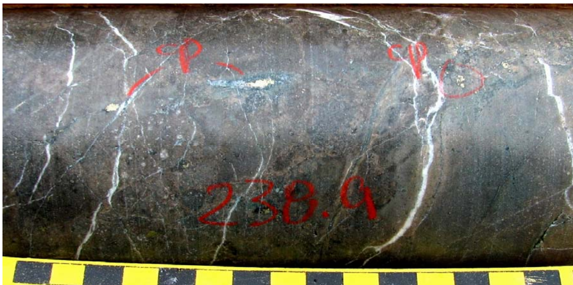
Fig 10-2-11: 06CF264-238.9 m. ANTF, Andesitic Tuff. The lower right portion shows a very fine grained, homogeneous tuff with weak bedding. The left part of the photograph shows a fine grained, clastic tuff with mm lapilli. Note the disseminated chalcopyrite throughout the sample.
