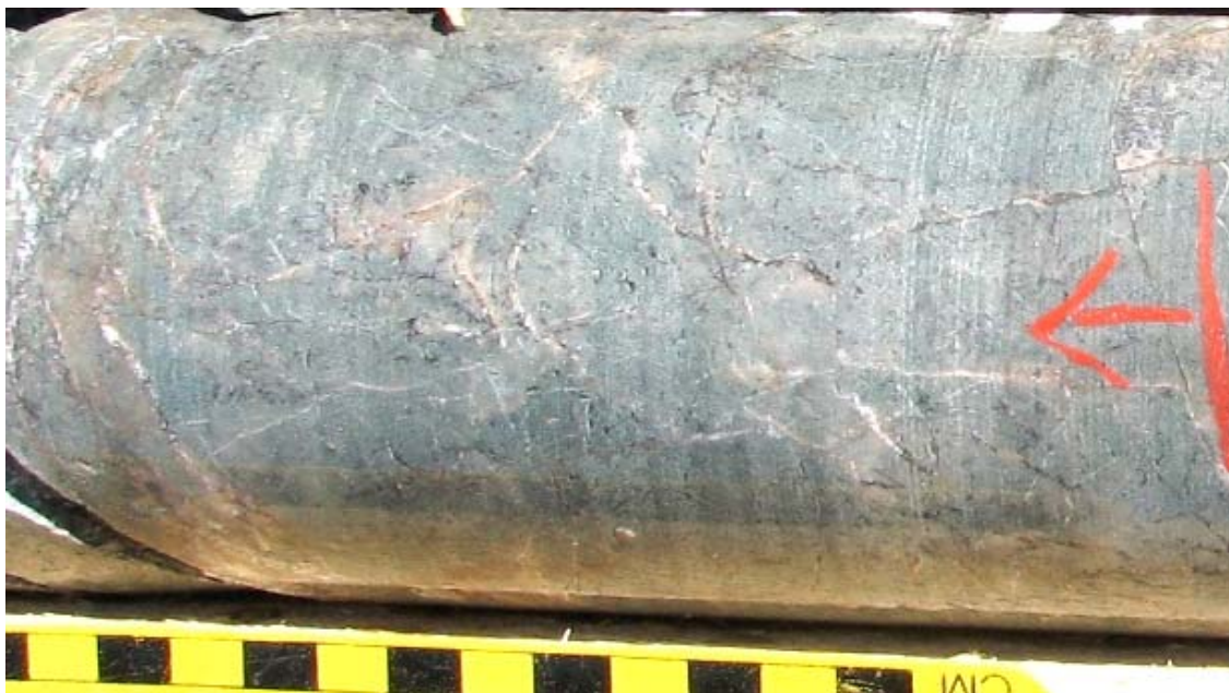
Fig 10-2-15: 06CF249-122.0 m. ANDS, Andesite. A massive, very fine grained to aphanitic, igneous lava of intermediate composition with no discernible phenocrysts.
