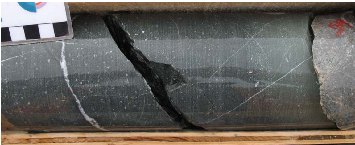
Fig 10-2-1: 06CF284-58.8 m. D/BS, Basic Dike. Massive, feldspar phyric mafic dike with chilled margin at contact to feldspar phyric andesite, shown on the right.
