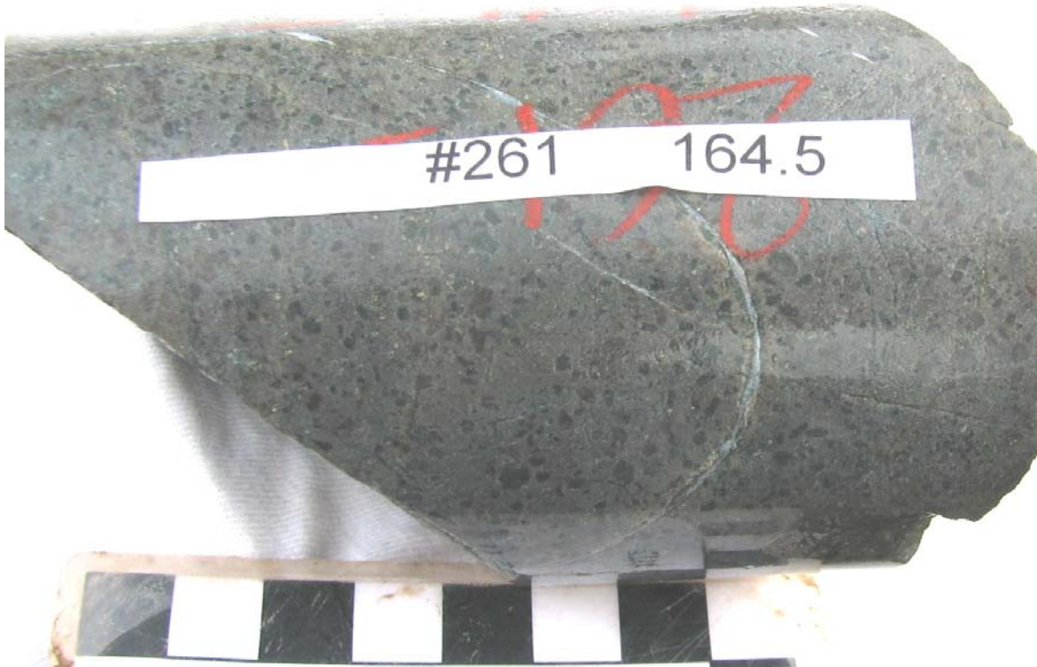
Fig 10-2-19: 06CF261-164.5 m. ANAU, Augite Phyric Andesite. Subhedral, altered, dark green augite phenocrysts, 1-2 mm in size, within a weakly altered, fine grained, igneous groundmass. The augite phenocrysts are entirely replaced mainly by chlorite.
