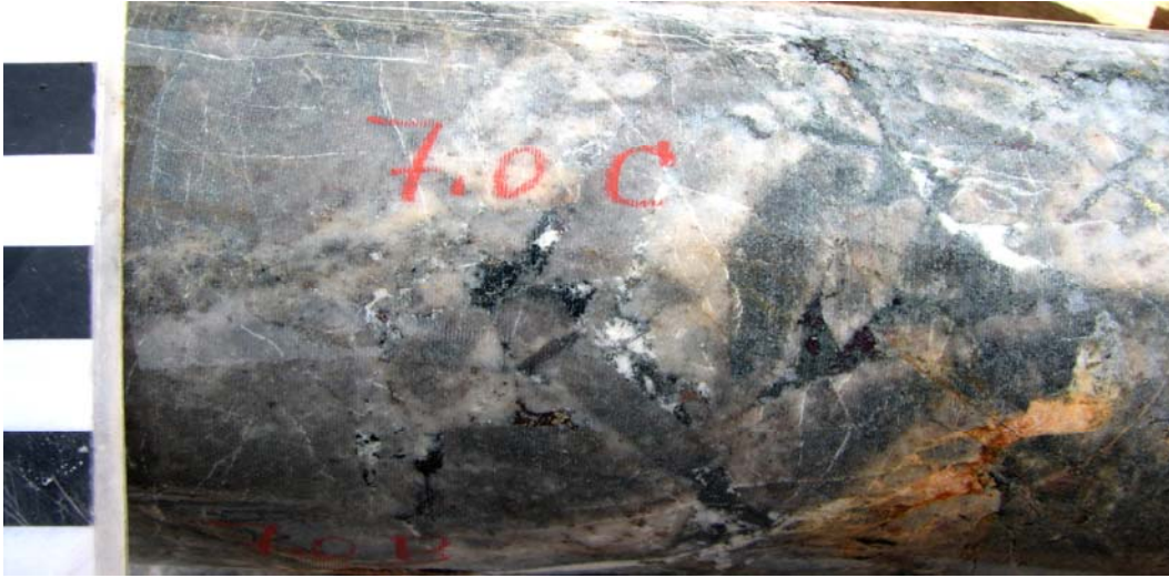
Fig 10-2-10: 06CF288-7.0 m. BRIG. Intrusive – Hydrothermal Breccia. Angular clasts of grey feldspar porphyry in 20 % igneous breccia matrix of light grey, fine grained, feldspathic rock. Subsequent hydrothermal infilling by chlorite, bornite, pyrite and carbonate.
