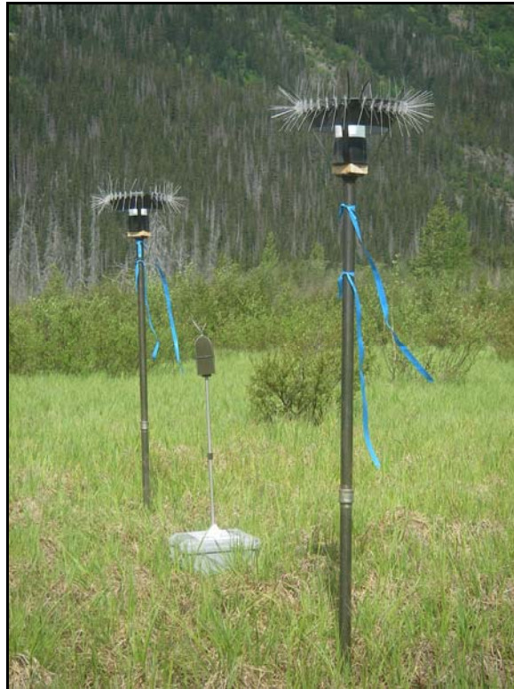
Plate 2-1. Photograph of a Quest Model 2900 sound level meter (centre) at Schaft Creek station FD-7 surrounded by two dustfall collectors
