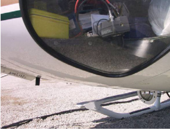
Figure 9. Digital video camera typical mounting location.
