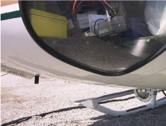
Figure 9. Digital video camera typical mounting location.
