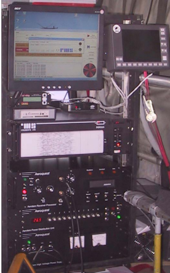
Figure 8. AeroTEM II Instrument Rack., including AeroDAS and RMS DGR-33 systems, AeroTEM power supply, data acquisition computer and AG-NAV2 navigation system.
