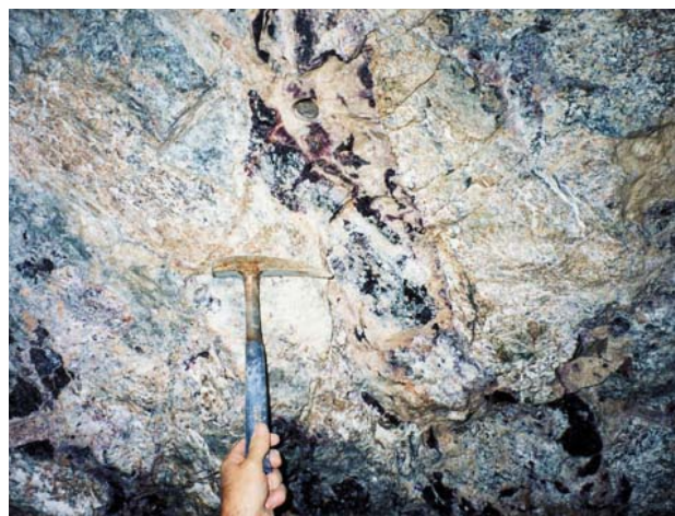
Figure 16. Mineralized breccia in adit 2 of the Eaglet property, showing patchy purple fluorite, flesh-coloured veins of K-feldspar, white celestite and blue-grey silicified zones.
