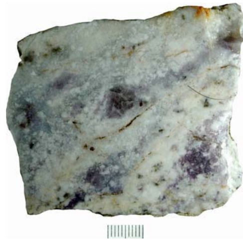
Figure 18. Typical fluorite (FI) – celestite (ClS) – quartz (Qtz) mineralization from adit 2, Eaglet property. Sample is 5 cm across.
